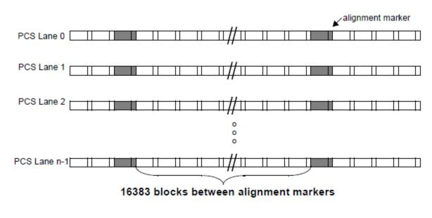
Figure 82-8—Alignment marker insertion period
