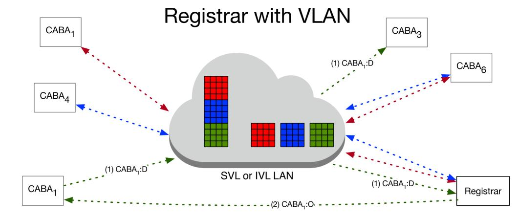
Network is configured with Registrar on all active VLANs on which BARC is used.
