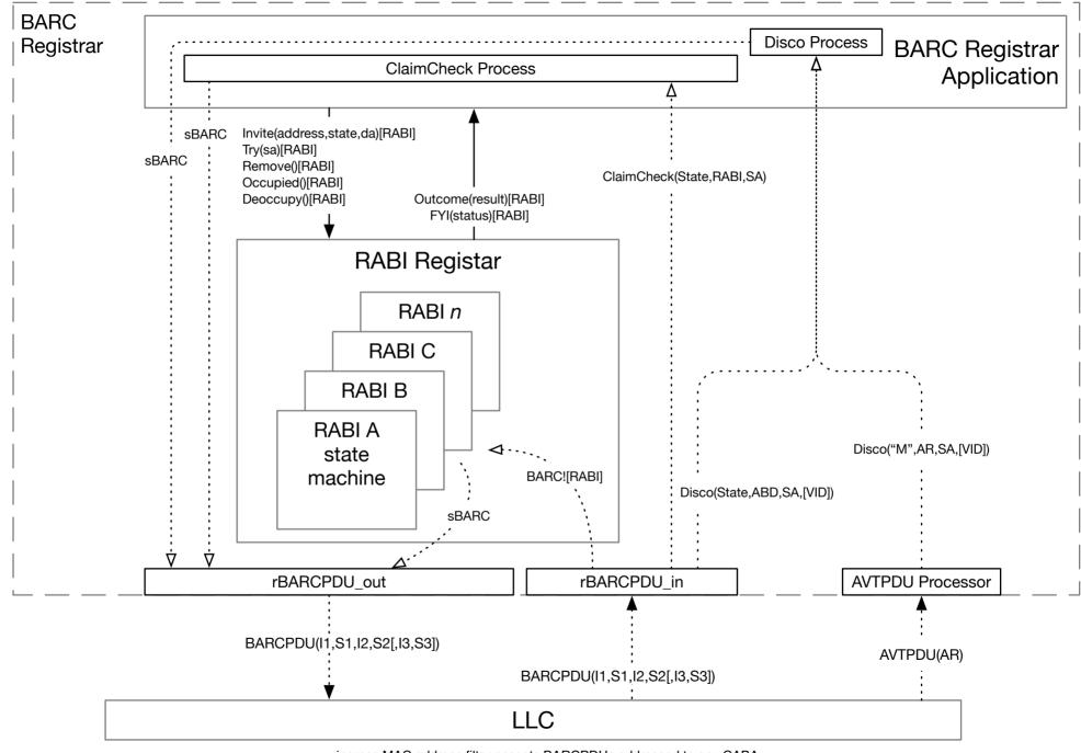
ingress MAC address filter accepts BARCPDUs addressed to any CABA and MAAP multicast address for AVTPDUs
