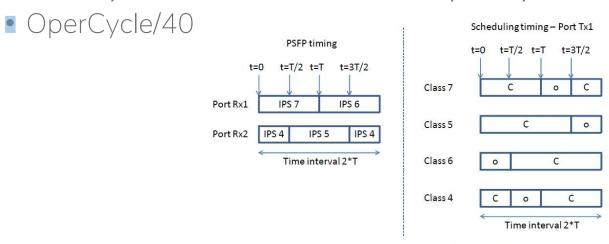
Figure T-5—Interleaving example—factor of 2
