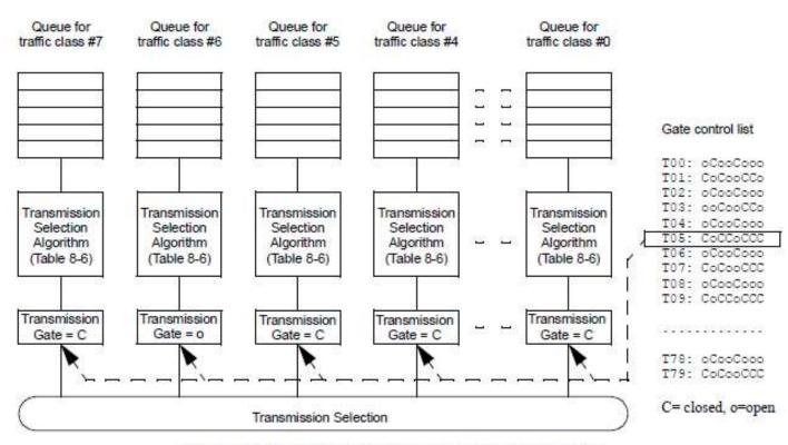
Figure 8-16—Transmission selection with gates
