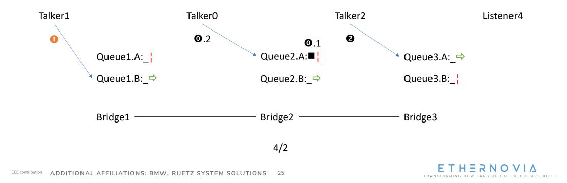
Guard-Band Start on Queue3.A! Queue1.A can open up after Tolerance-Band!
