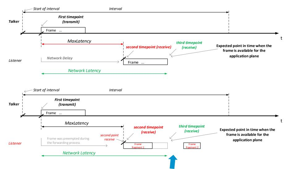
In case of preempted packets (and the AccumulatedLatency=MaxLatency), with the actual "MaxLatency" definition, it is not possible for the listener to derive the worst-case point in time when the stream's frame is fully received, i.e. the point in time when the internal processing starts. The CNC and the listener needs to do additional translations
