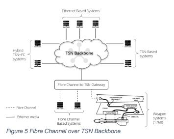
The Fibre Channel based systems may include legacy equipment (such as data storage, sensors, displays, DSP processors, etc) as well as interfaces to next generation stores (via a high speed 1760 interface). The architecture includes an option for hybrid systems that include a mixture of TSN and Fibre Channel (i.e. Ethernet end systems that implement Fibre Channel upper layer protocols and communicate with other Fibre Channel based systems).
