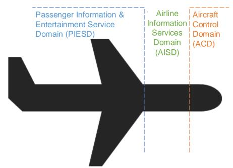
The Aircraft Control Domain (ACD) networks host equipment that contribute to the safe flight of the aircraft. Functions typically hosted on the ACD network include electronic flight instrument system (EFIS), engine-indicating and crew alerting system (EICAS), flight management system (FMS), flight controls, and other control systems. Due to the high criticality of the functions hosted, the ACD network has high safety requirements and deterministic behavior is required.
