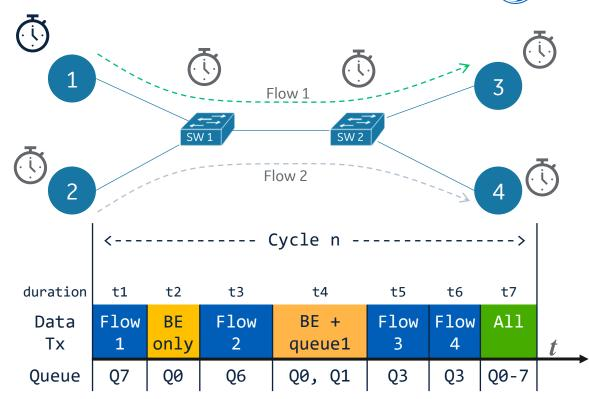
Gate Control List for the above schedule at a given egress port: OCCCCCC t1 CCCCCCO t2 COCCCCC t3 CCCCCOO t4 CCCOCCC t5 CCCOCCC t6 OOO0000 t7
