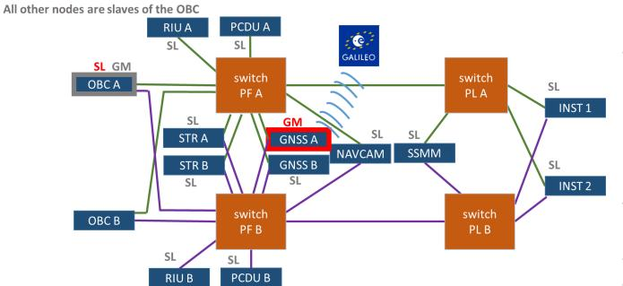
In addition to providing the PVT acquisition to the OBC, the GNSS offers a synchronization service to the network. Failure and reconfiguration to the redundant GNSS would lead to a synchronization loss. Indeed, GNSS takes one minute (order of magnitude) after switch-on to be able to provide the synchronization service.
