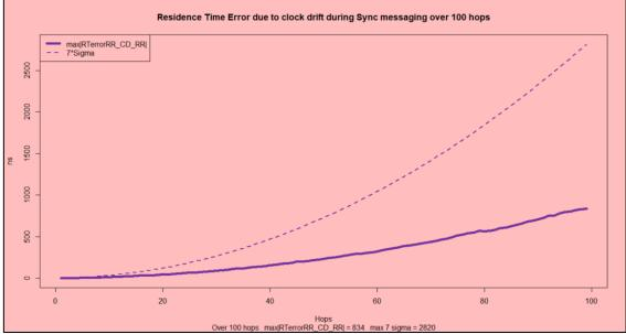
Algorithmic Compensation for Error Due to Clock Drift During Sync Messaging
