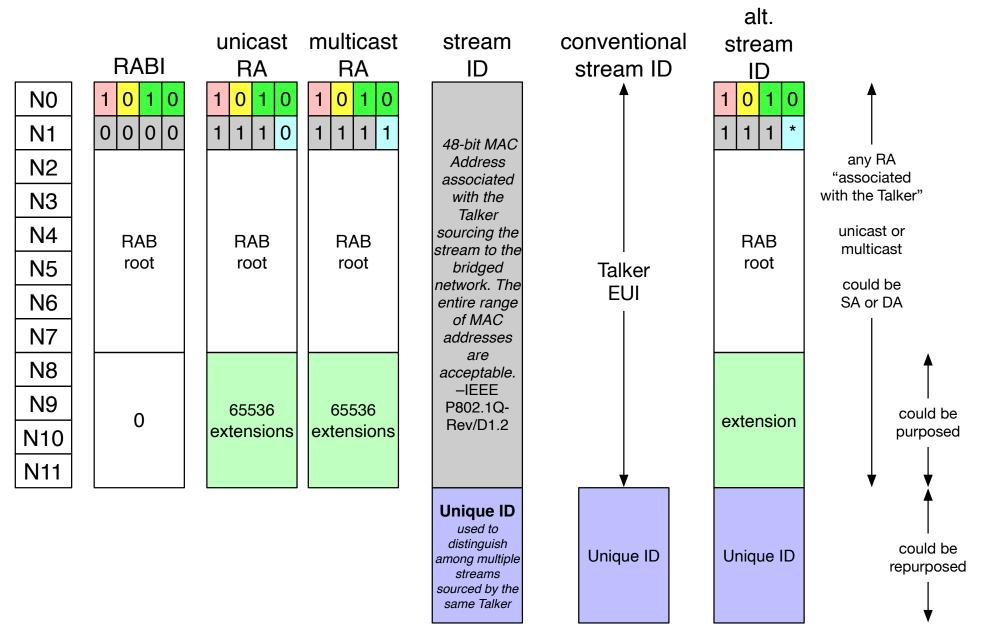
The MAC address component of the StreamID can, but does not necessarily, have the same value as the source\_address parameter of any frame in the actual data stream.
