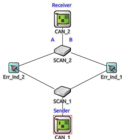
Figure 5: Seamless CAN setup in failover simulation scenario.
