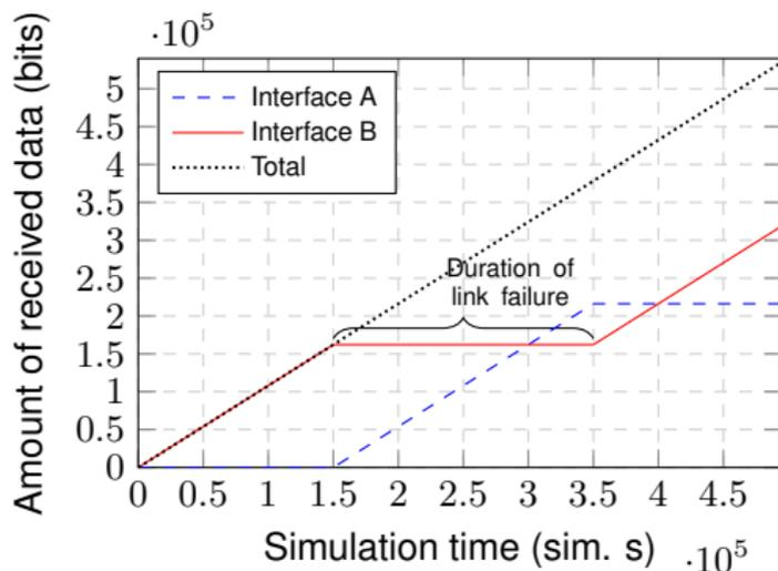
Figure 6: Seamless CAN frame reception performance in the case of link failure.
