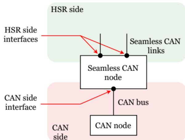
Figure 3: Seamless CAN node's interfaces.
