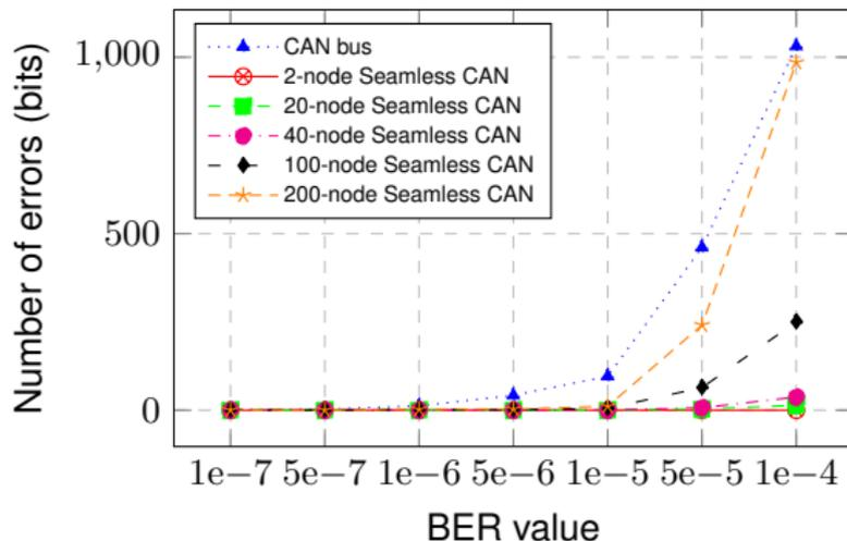
Figure 7: Seamless CAN network's bit error results in comparison with CAN bus with different BER values and numbers of nodes.
