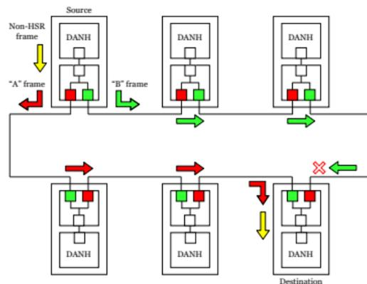
Figure 1: Example of an HSR ring.
