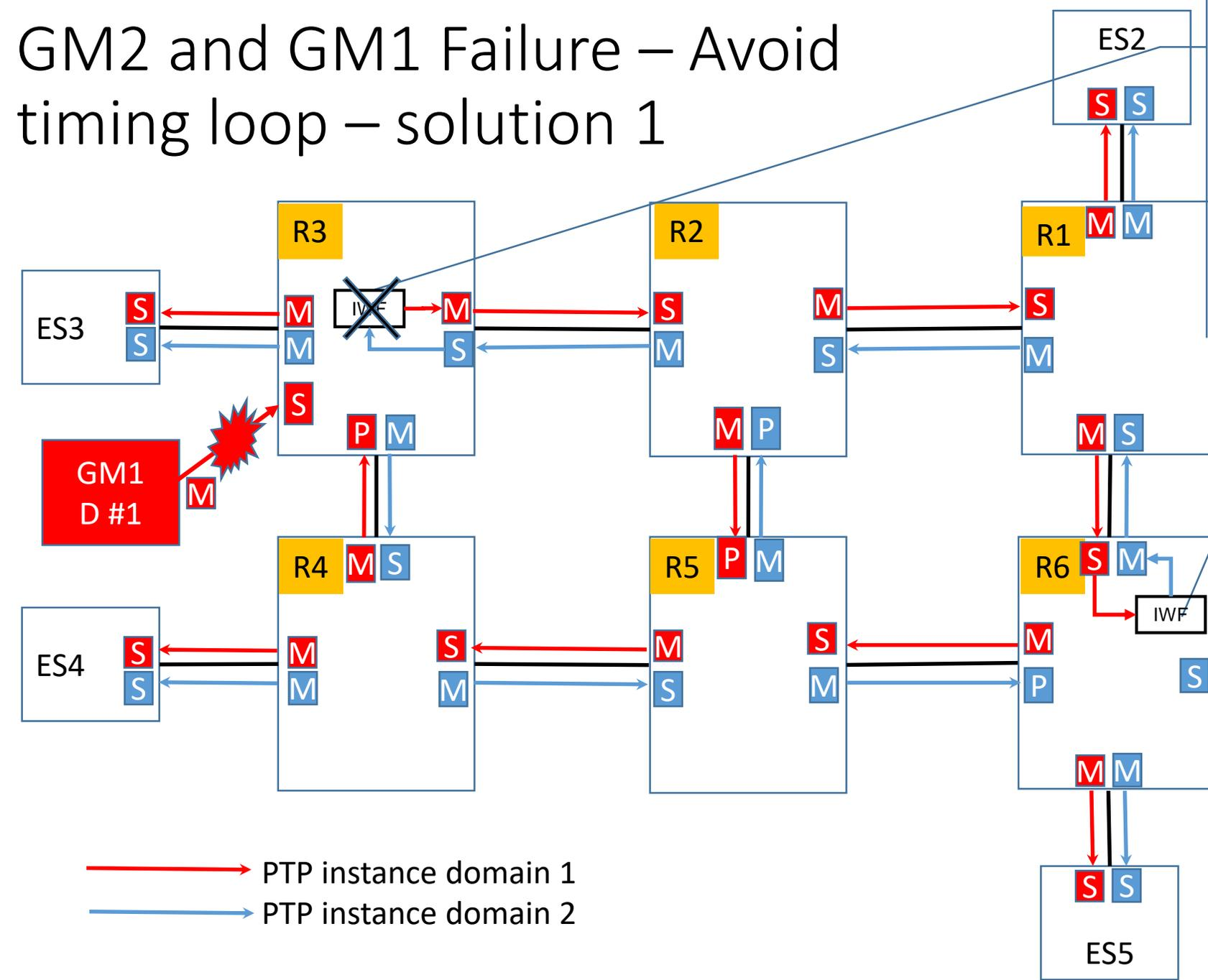
When GM1 fails, R3 knows that it should not activate the IWF as Domain 2 was using the time from Domain 1, **because it does not receive Announce message from the GM of Domain 2**, and therefore this information can be used to avoid the timing loop.
