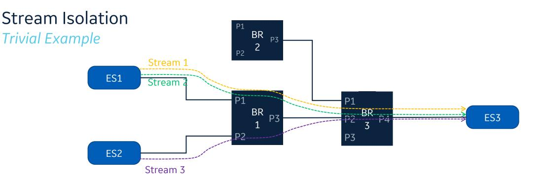
**Option 1:** Isolating failure (misbehaving) of streams, end-stations, and bridges requires policing of all streams at each hop.
