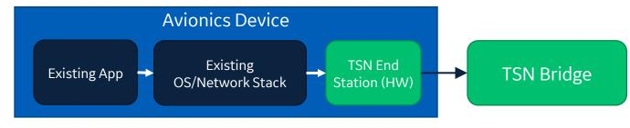
The existing stack will fully assemble the frame. Assuming the integrator has established L2/L3 addressing conventions, those headers will need to transform to comply with the Integrator network conventions.
