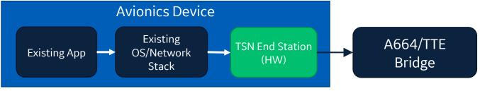
Existing stack will fully assemble the frame. The L2 & L3 headers must be transformed by the TSN End Station to comply with the Integrator network conventions.
