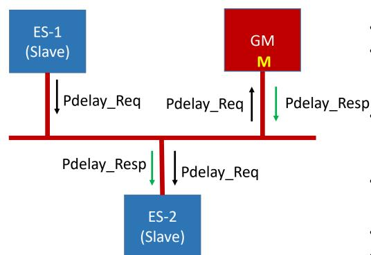
Note that if Announce message is not used, then Sync message can still be used to identity the GM clockID, even though sourcePortIdentity field of the PTP common header identifies the upstream master port, which, in this case, is the GM.
