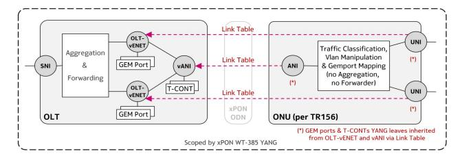
The ONU's 'UNI' at the right side of this picture can be an Ethernet interface. We want to make it possible that in some networks the connected equipment shall use the 802.1X protocol for port-based authentication. Then logically the ONU should support 802.1X on these Ethernet interfaces. However, most existing ONU do not support the 802.1X protocol.
