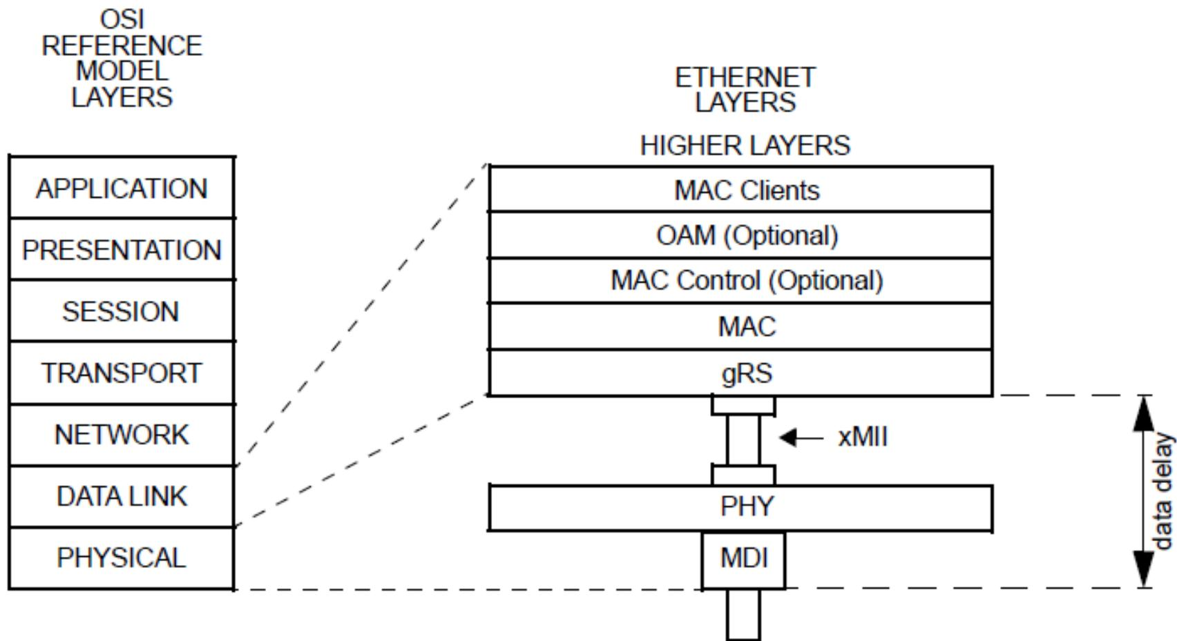
**Figure 90-5—Data delay measurement**
