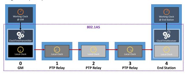
The Monte Carlo simulation covers only the portion of the diagram in the "802.11AS" box. At the GM it effectively assumes that the Working Clock @ GM is the same as the Local Clock @ GM. At the End Station it only models the (unfiltered) output of the ClockTimeReceiver.
