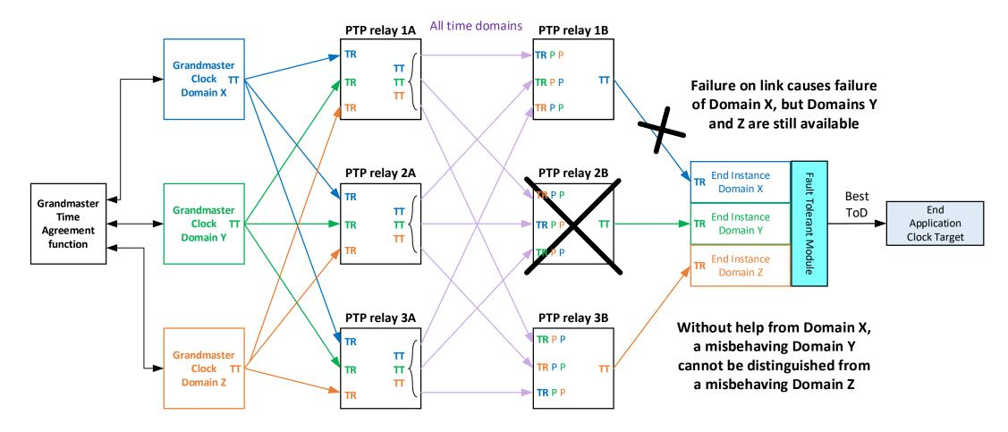
After one failure, this End Application is "fail stop" (i.e., another failure can be detected, but cannot be overcome)
