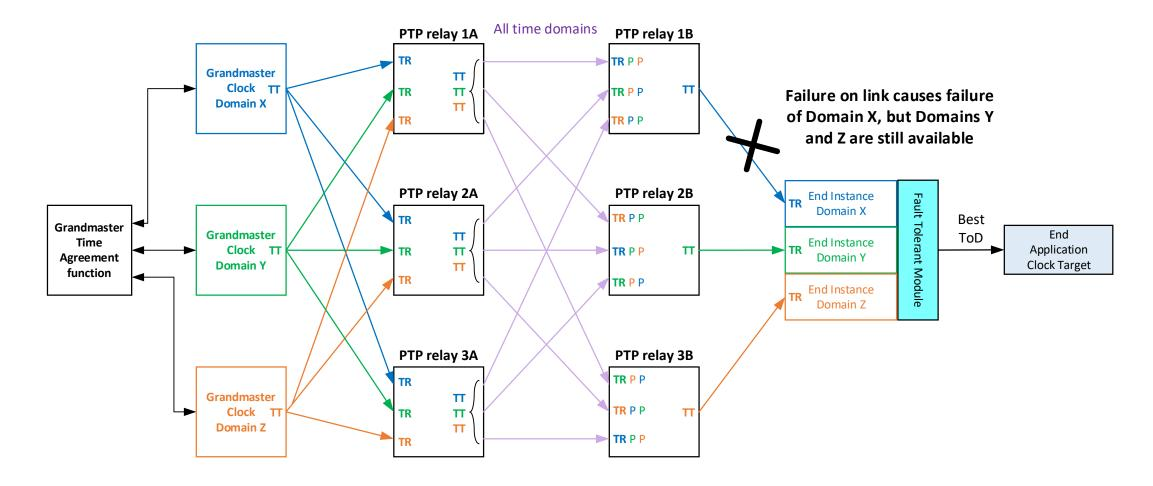
• End Application is "fail operational" (i.e., can still operate properly after 1 failure)
