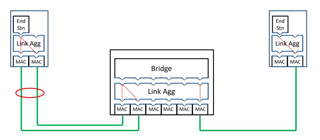
Link Aggregation Sublayer sits between Bridge Ports and MACs in a bridge; between MAC Client(s) and MACs in an end station.
