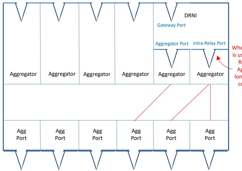
When an Aggregator is used for the Intra-Relay Port, that Aggregator is no longer available to connect up to a bridge port.
