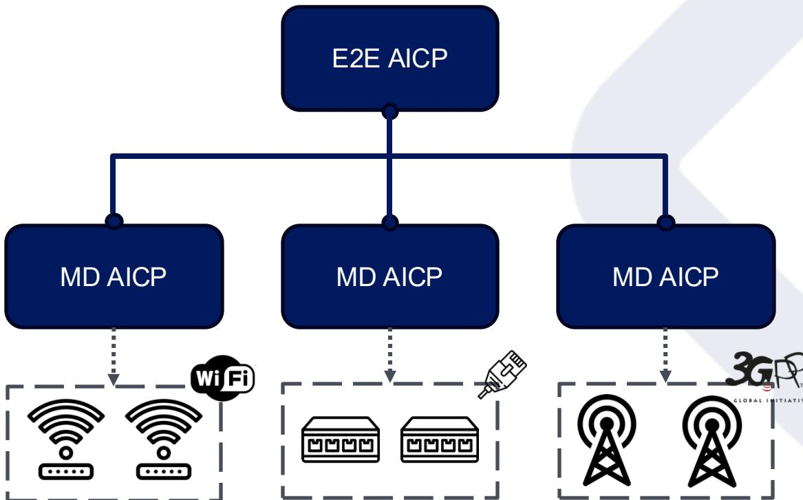
The AICP Architecture is divided into End-to-End (E2E) AICP and Management Domain (MD) AICP:
