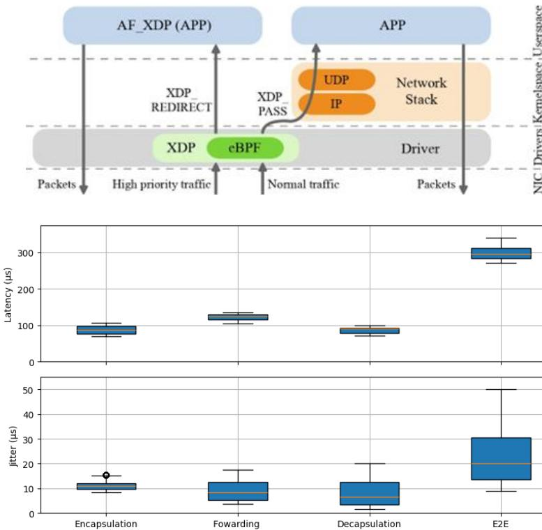
Fully open-source, programmable DetNet router on Linux using XDP and eBPF
