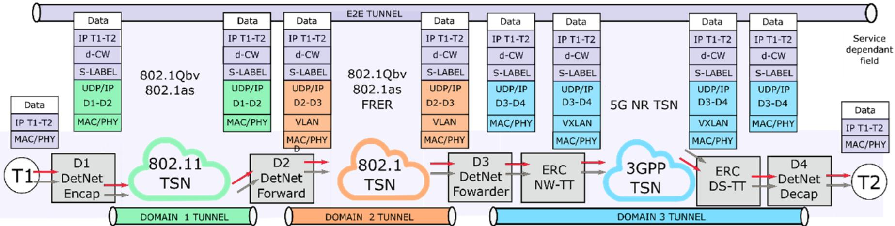
MPLS-encapsulation spans Wi-Fi TSN → Ethernet TSN → 3GPP 5G TSN, preserving flow identity and timing metadata
