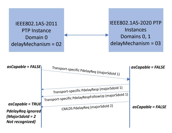
1. What is the definition of Backward Compatibility? Our Expectation: Pair any IEEE802.1AS-2020 implementation with any IEEE802.1AS-2011 – expect IEEE802.1AS-2020 to step down to IEEE802.1AS-2011 'mode' of operation (transmit Pdelay **Request messages with** MajorSdold set to 1; set delayMechanism to 02) 2. Is this a valid test? 3. Or should the test setup configure
