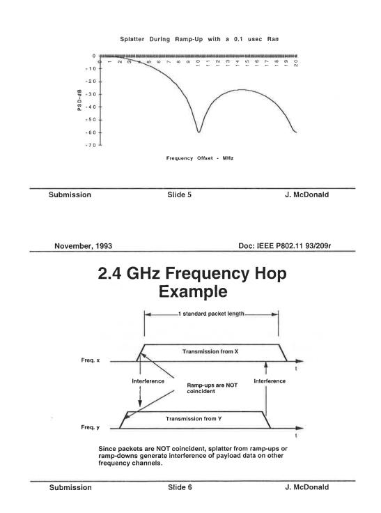
Splatter with 0.1 usec Ramp-Up
