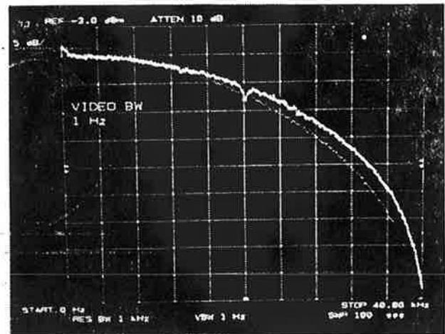
Figure 7(b). Picture of Baseband Power Spectral Densities after Gaussian,  $BT_b=0.5$  Filter (thin curve, DECT-Chip LMX2411; 9 samples/bit; 8 bits resolution) and FQPSK-1 Baseband Filter (light curve, XILINX-FPGA; 8 samples/bit; 8 bits resolution) at normalized scaled down bit rate of 40kb/s (measurements were also done at 1Mb/s).
