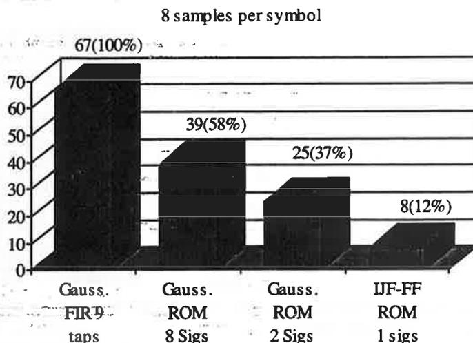
Figure 5. XILINX-FPGA Gate Count Comparison in numbers of packed CLB's for several Filter Implementations.
