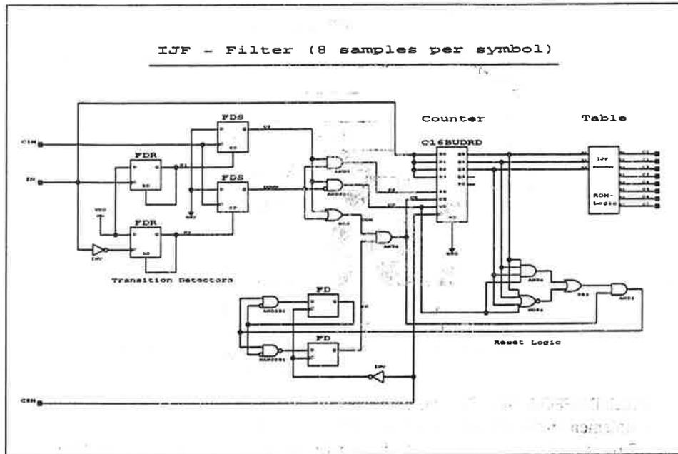
Figure 4. Schematic for the XILINX-FPGA Implementation of ROM Look-up Table based FQPSK-1 Baseband Filter with 8-samples per data bit, 1 bit signal length and 8-bit signal resolution. This design uses Feher's patented Filter structure [9] and reduces the number of packed CLB's by a factor of about 8 compared to the design Figure 3.
