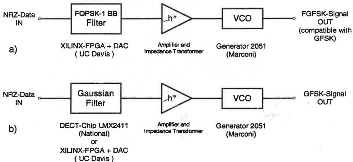
Figure 1. Block diagrams of compared FGFSK-(a) and GFSK-(b) modulator structures
