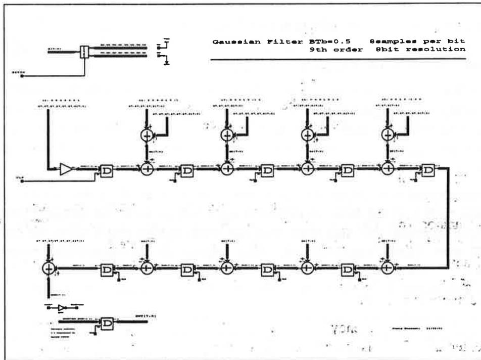
Figure 3. Schematic for the XILINX-FPGA Implementation of Gaussian,  $BT_b=0.5$  FIR-Filter with 8-samples per data bit, 9-tap impulse response length, and 8-bit signal resolution. The design is used for gate count comparison purposes and is based on [11].
