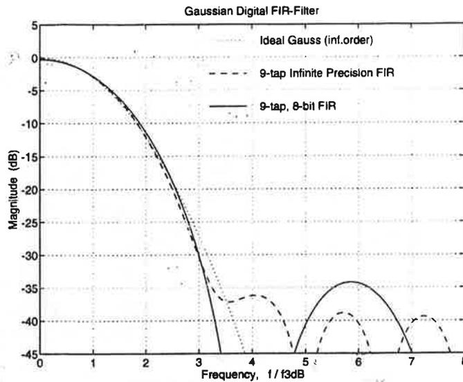
Figure 2. Frequency Response of Gaussian,  $BT_b=0.5$  FIR-Filter Approach with 8-samples per data bit, 9-tap impulse response length, and 8-bit signal resolution
