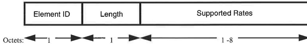
**Figure 4, Supported Rates Element Format**
