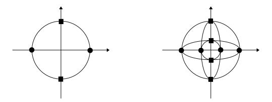
Fig. 1: Trajectories of MSK/OQPSK and OQAM
