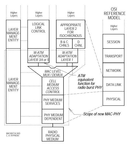
Figure 2 Protocol Stack for New ISLAN with MAC Level Multiplexing
