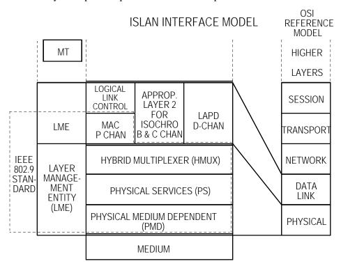
Figure 1 IEEE 802.9 Protocol Stack with Phy Multiplexing of Integrated Services
