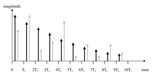
Fig 1: Channel impulse response; black illustrates average magnitudes, gray illustrates magnitudes of a specific random realization of the channel; the time positions of black and gray samples are staggered for clarity only.
