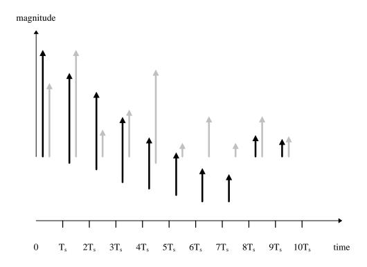
Fig 1: Channel impulse response; black illustrates average magnitudes, gray illustrates magnitudes of a specific random realization of the channel; the time positions of black and gray samples are staggered for clarity only.
