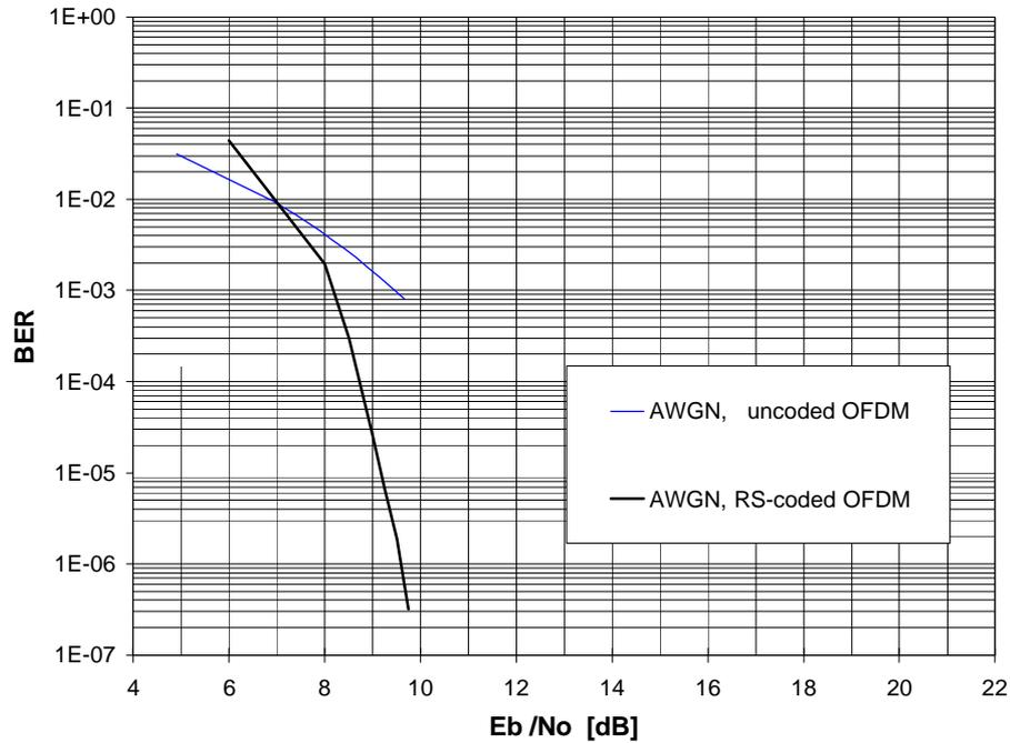
Figure 10: Uncoded and coded bit error rates of the overall MEDIAN physical layer in AWGN (comparable to demonstrator). HPA nonlinearities, LO phase noise, synchronisation are included.
