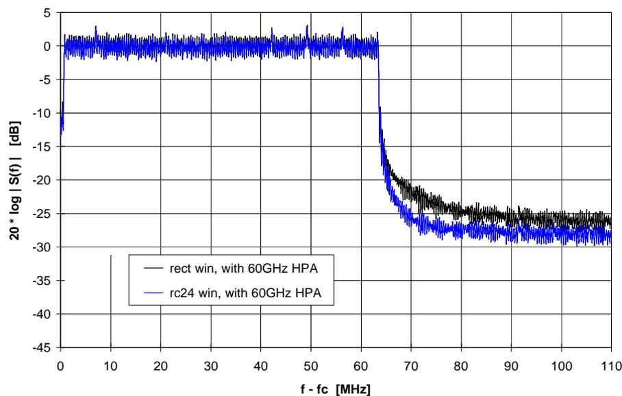
Figure 9: Power spectral density of OFDM modulated transmit signal for 2 types of Tx-windowing (rectangular and raised cosine roll off, see sect 3.5) after 60GHz high power amplifier (demonstrator HPA, Figure 6, 5dB OBO with respect to 1dB compression point).
