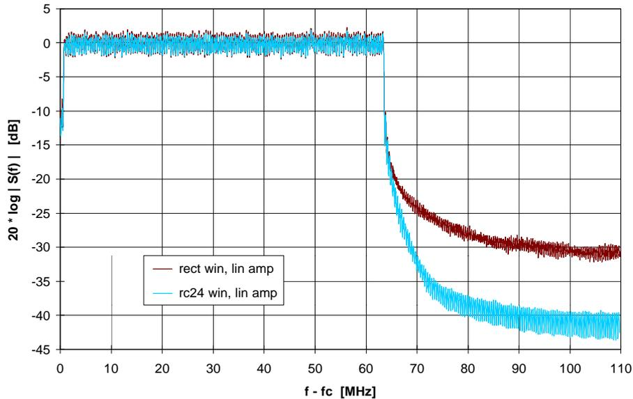
Figure 8: Power spectral density of OFDM modulated transmit signal for 2 types of Tx-windowing (rectangular and raised cosine roll off, see sect 3.5) after linear amplification.
