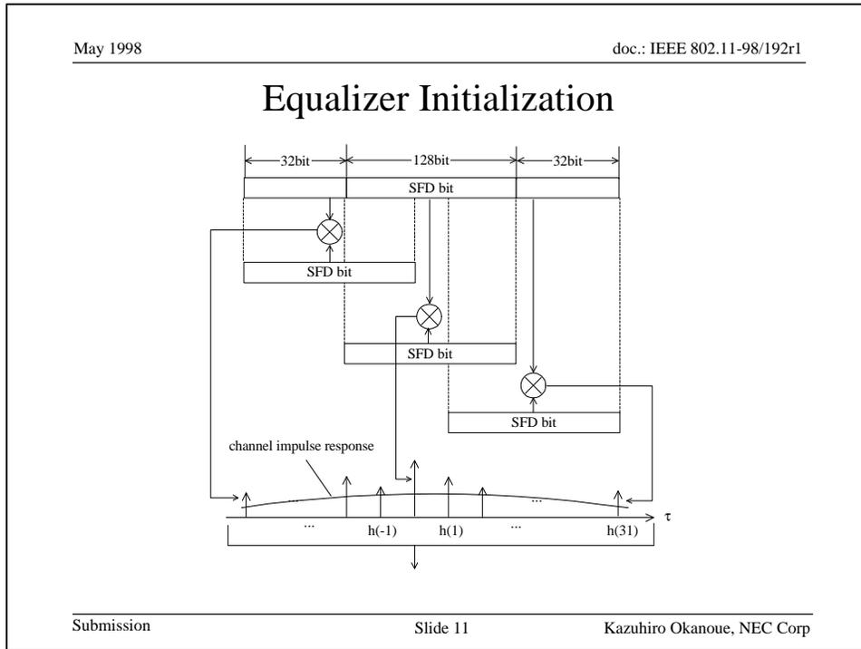
The MLSCE requires only channel impulse response for its initialization. In order to estimate channel impulse response, a correlation technique between received signal and known preamble sequence can be available as shown in this slide.
