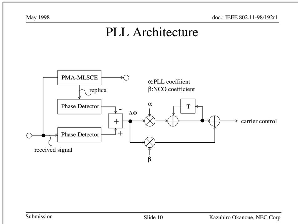
In order to obtain stable carrier, we use 2<sup>nd</sup> order PLL by using PMA-MLSCE output and received signal. The PMA-MLSCE calculates replica of received signals. A phase difference between received signal and a replica which produces minimum metric is input to the 2<sup>nd</sup> order PLL. The PLL output controls carrier frequency and phase.
