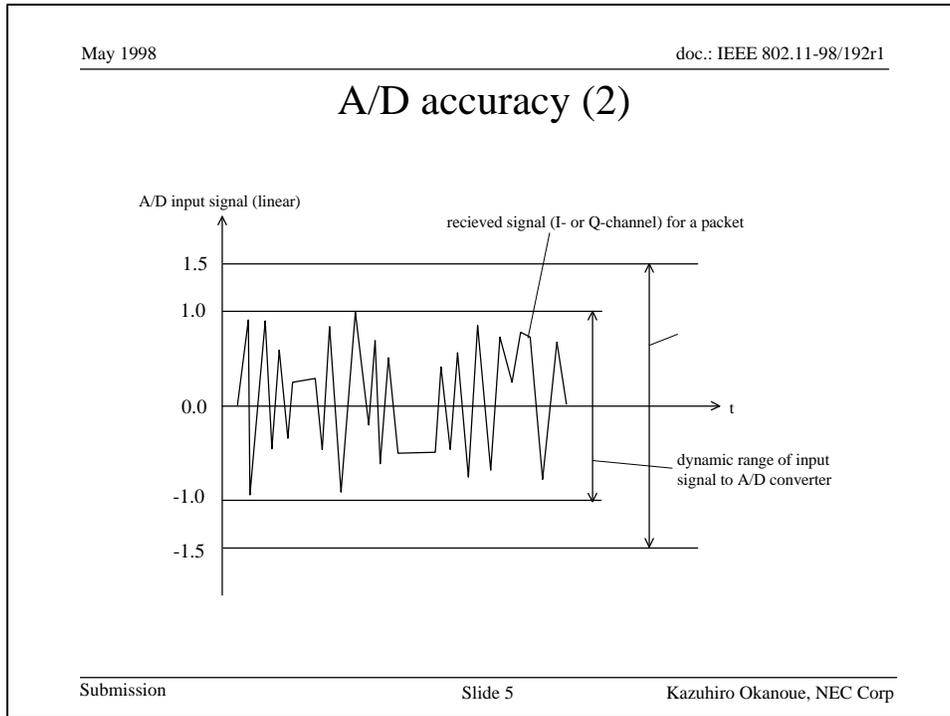
In the simulation, I assumed a dynamic range of input signal level as +/- 1.0 and a dynamic range of A/D converter as +/- 1.5, as shown in this slide.
