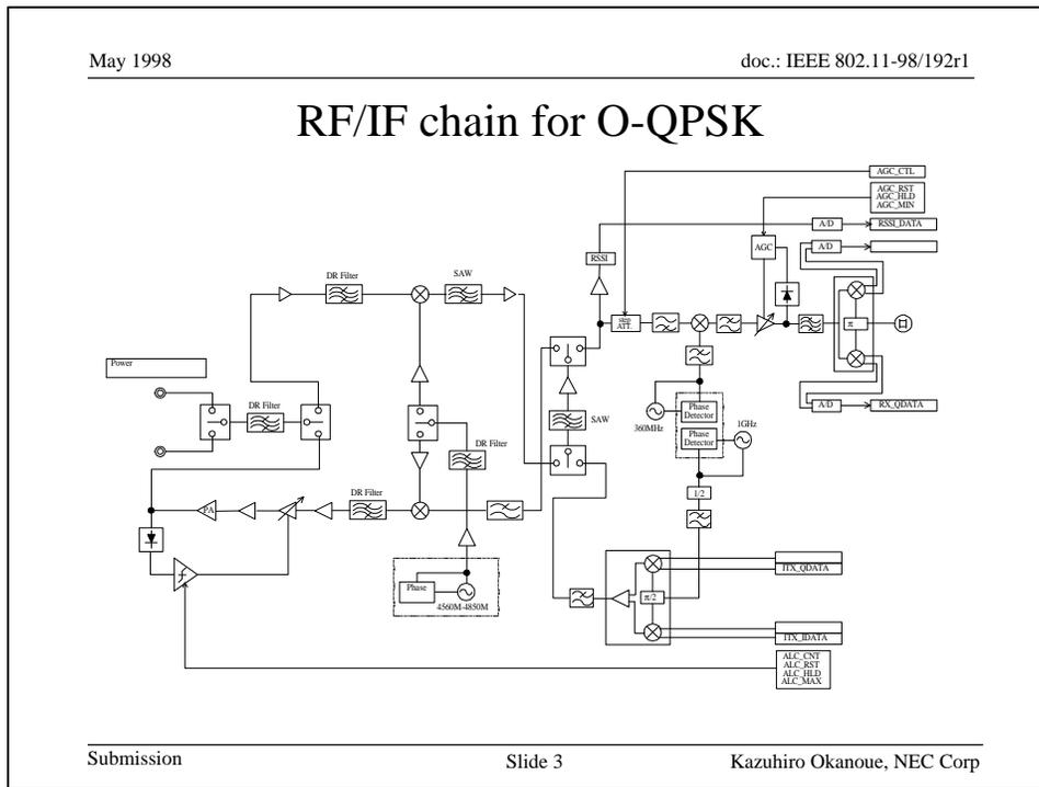
This slide shows an example implementation of RF/IF chain for O-QPSK.
