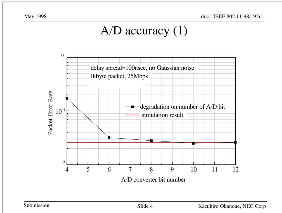
This slide shows a packet error rate (PER) performance vs A/D accuracy in an environment of 100nsec delay spread. This figure indicates that A/D accuracy of 8-bit slightly degrades PER and the degradation seems to be negligible.
