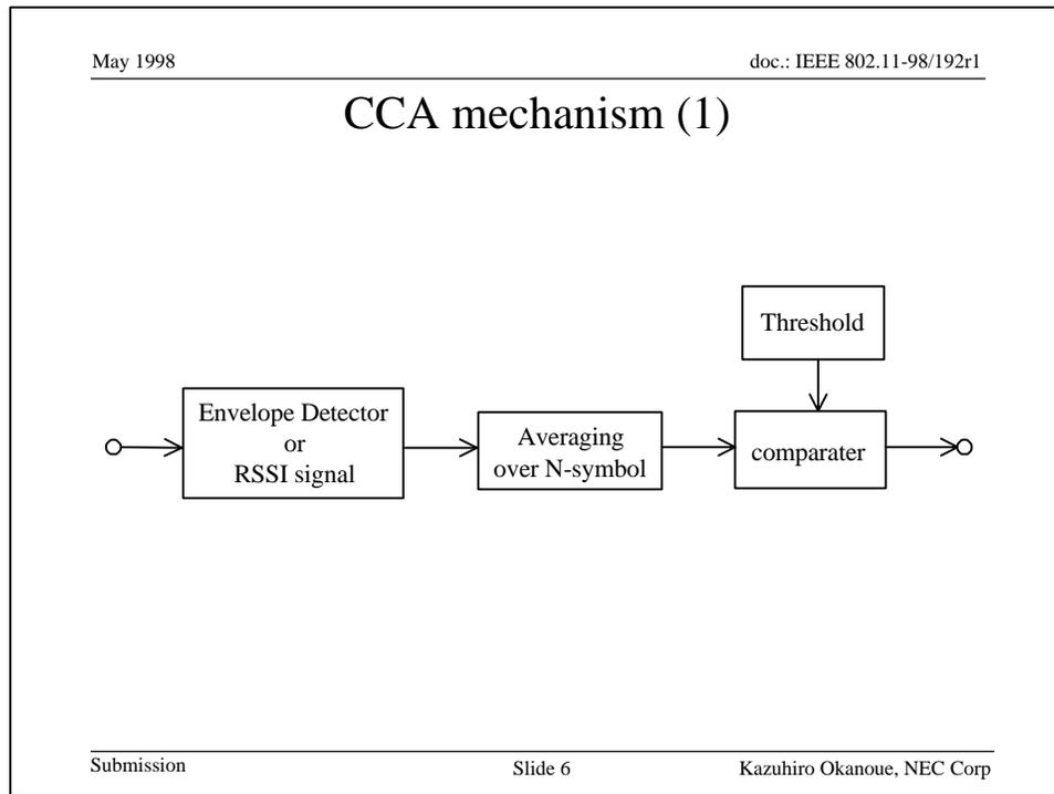
As a CCA detection mechanism, we propose to adopt envelope or RSSI signal detection mechanism as shown in this slide. When an averaged envelope level of received signals gets over the threshold level, the CCA detector detects that the medium is busy.
