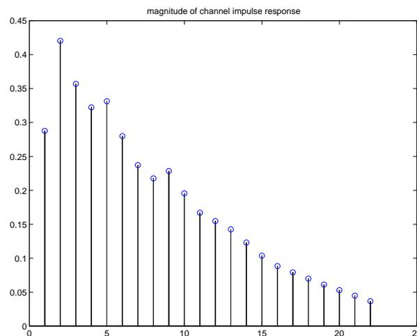
Figure 1: Channel amplitudes derived from C channel model
