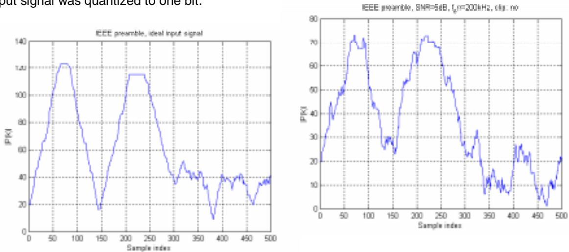
Figure 7: Output of the correlator device (Fig.6) with ideal and distorted signal with IEEE preamble.
