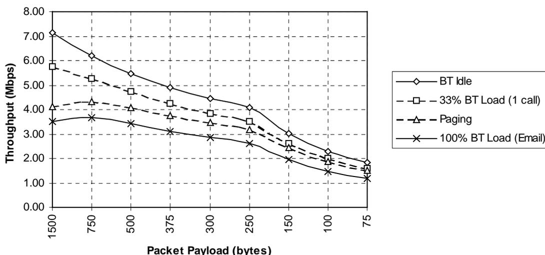
**Figure 3.2.1-2 Throughput for DSSS WLAN as a Function of Piconet Utilization (Single BT Interferer)**
