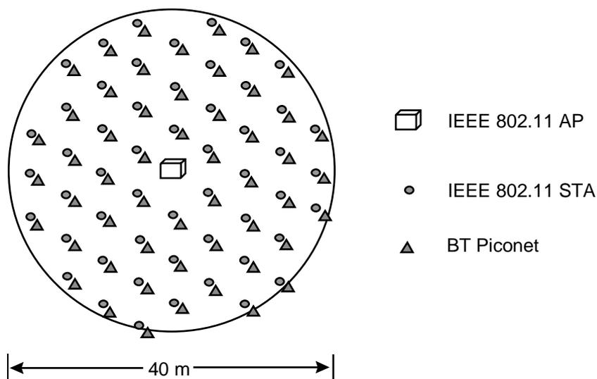
**Figure 2.2.1 Composite BT/DSSS Network Topology**
