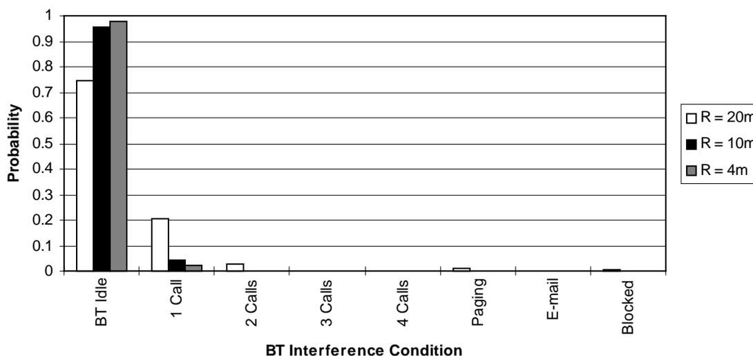
**Figure 5.0-1 BT Interference is Dependent on Range from AP**
