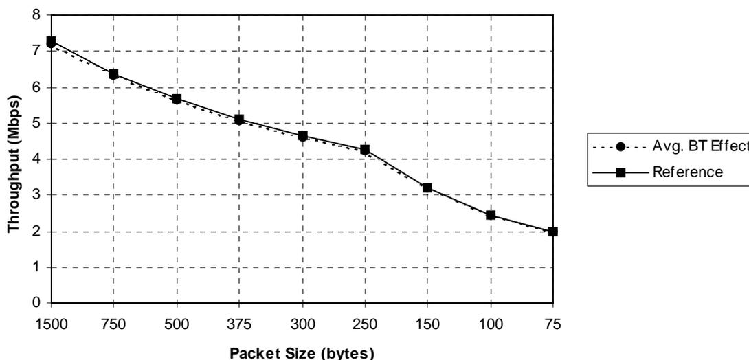
**Figure 4.3-1 Average Effect of BT Interference Over an 8 - Hour Day**
