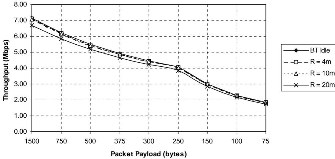
**Figure 5.0-2 IEEE 802.11 DSSS WLAN Average Throughput in Presence of BT Interference at Various Ranges from AP**
