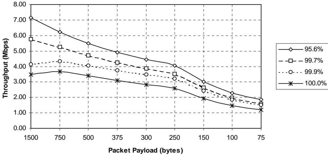
**Figure 5.0-4 Availability Curve for IEEE802.11 WLAN in Presence of BT Interference (Range to AP = 10 m)**
