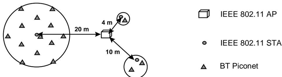
**Figure 3.1.1-1 Number of Potential BT Interferors Depends on Range from AP**
