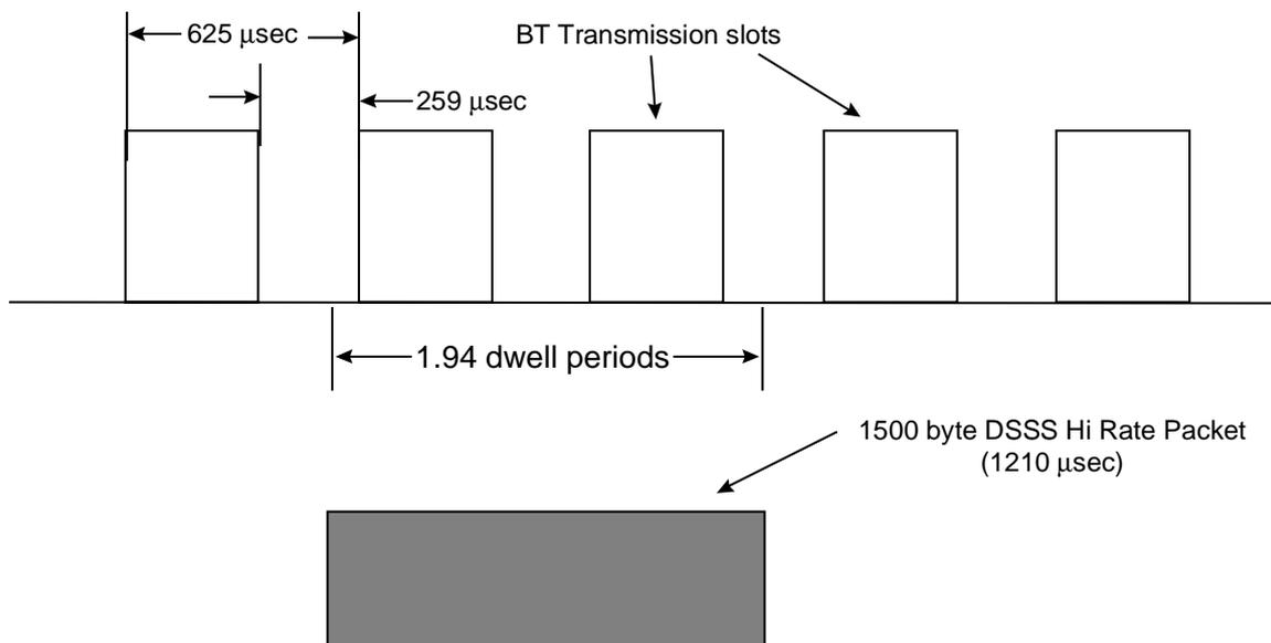
**Figure 3.2.1-1 Probability of Collision Depends on Number of BT Slots Overlapped**
