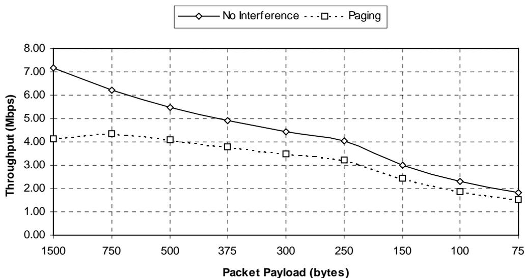
**Figure 4.1-2 IEEE 802.11 WLAN Throughput During BT PAGING Procedure**
