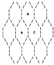
To move from one cell to the next cell, the moving station first contacts the next cell using the next cell's code at Aloha time. When a moving station leaves a cell that was supporting local traffic to the moving station then throughput can double, since one cell can devote all of its time to receive and the next cell can devote all of its time to transmit (or vice-versa).
