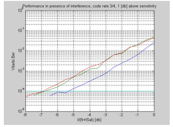
Remarks: Ber represent Ber at the Viterbi output. Threshold is set according to RS decoder threshold
