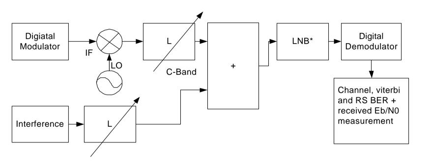
\*LNB sets the initial noise level. Interference is added on top.
