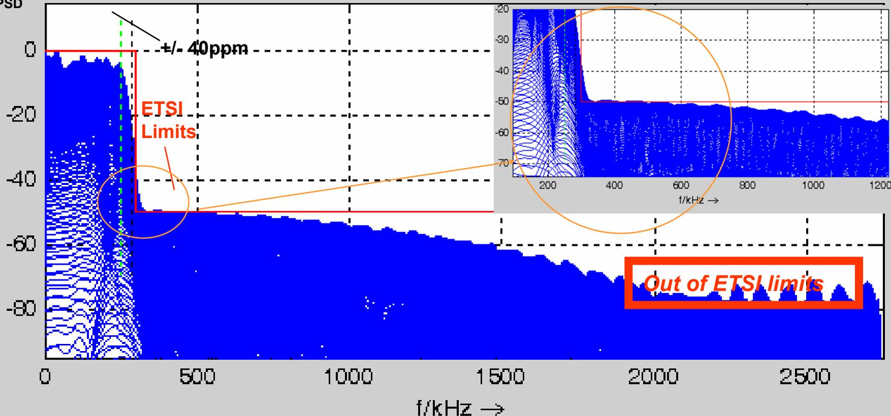
Simulations of the relative PSD in dB for the Cobi at 500 kchip/s, 250 kbit/s,  $r = 0.2$ ,  $\pm 40$  ppm.
