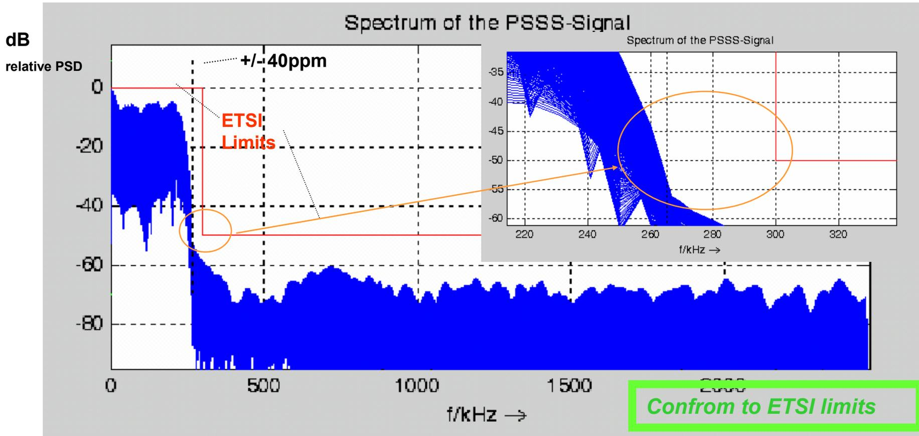
Simulations of the relative PSD in dB for the PSSS signal at 450 kchip/s 210 kbit/s,  $\pm 40\text{ppm}$
