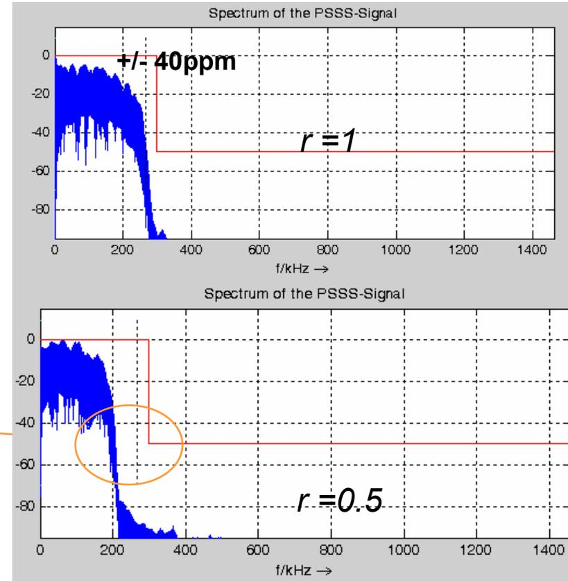
Simulations of the relative PSD in dB for the PSSS signal at 266 kchip/s 250 kbit/s.
