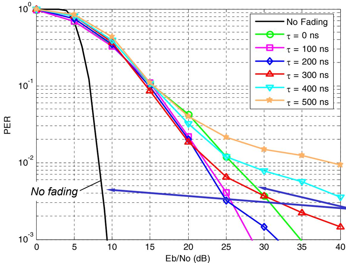
*Channel with 0ns RMS delay spread differs from "no fading" due to channel model characteristic*
