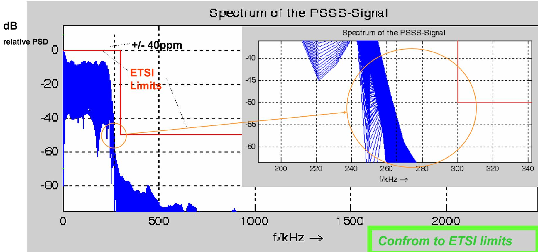
Simulations of the relative PSD in dB for the PSSS signal at 450 kchips/s, 210 kbit/s,  $\pm 40\text{ppm}$ .
