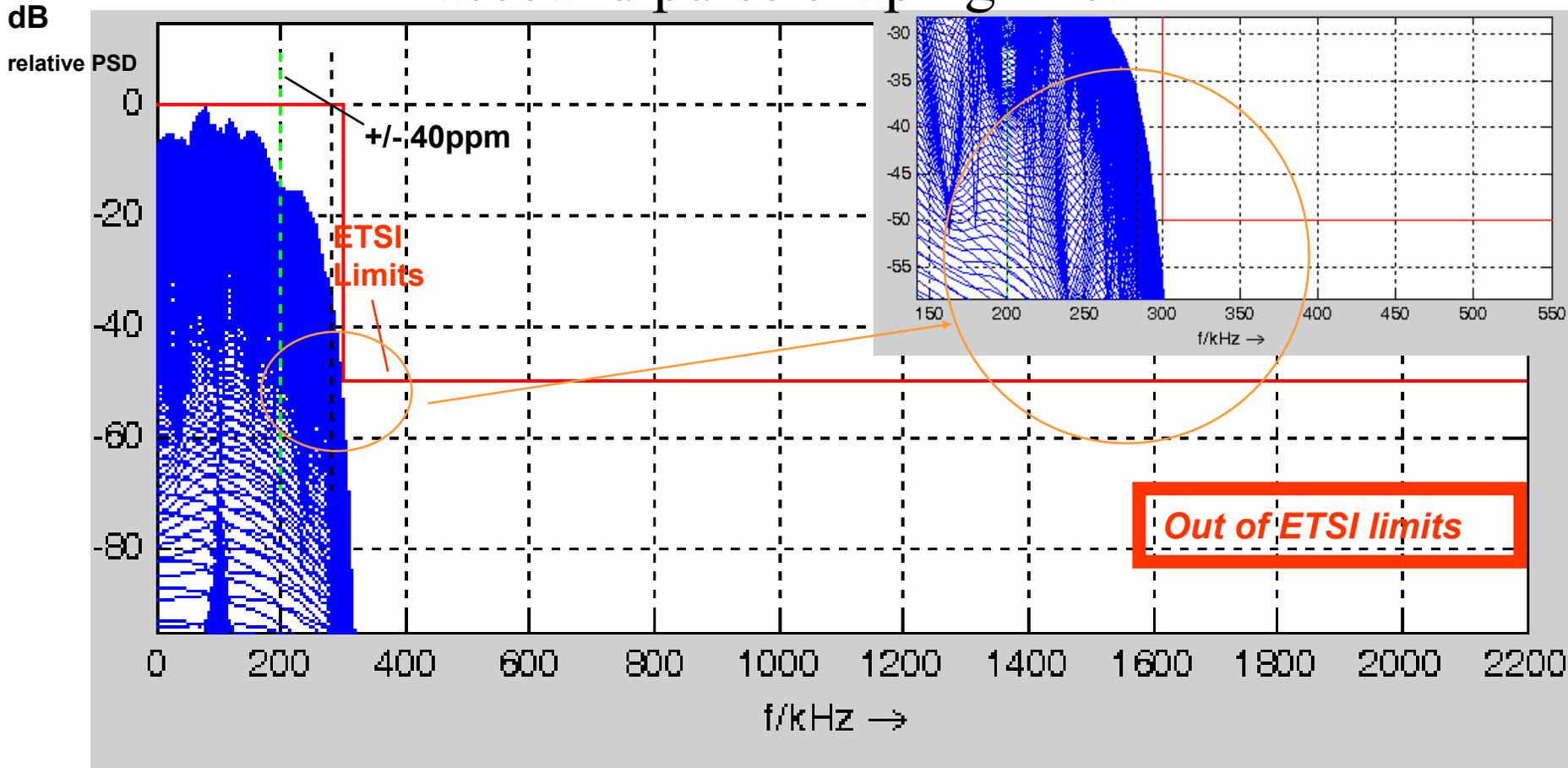
Simulations of the relative PSD in dB for the Cobi at 400 kchip/s, 200 kbit/s,  $r = 0.5$ ,  $\pm 40$  ppm.
