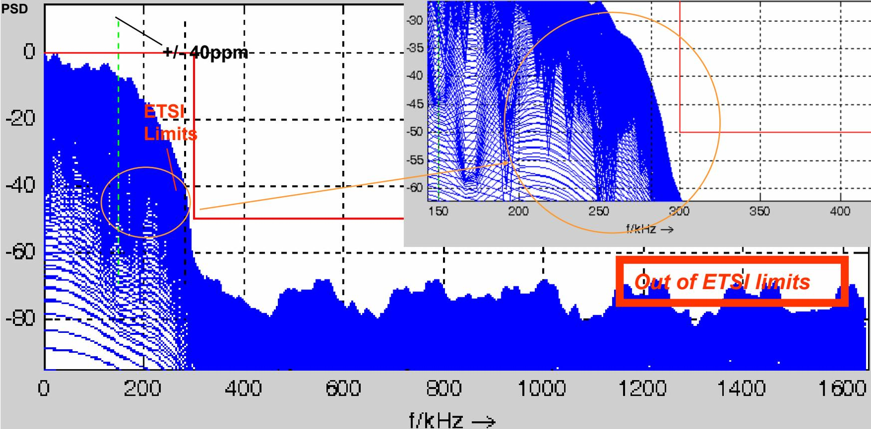
Simulations of the relative PSD in dB for the Cobi at 300 kchip/s, 150 kbit/s,  $r = 1 \pm 40$  ppm.
