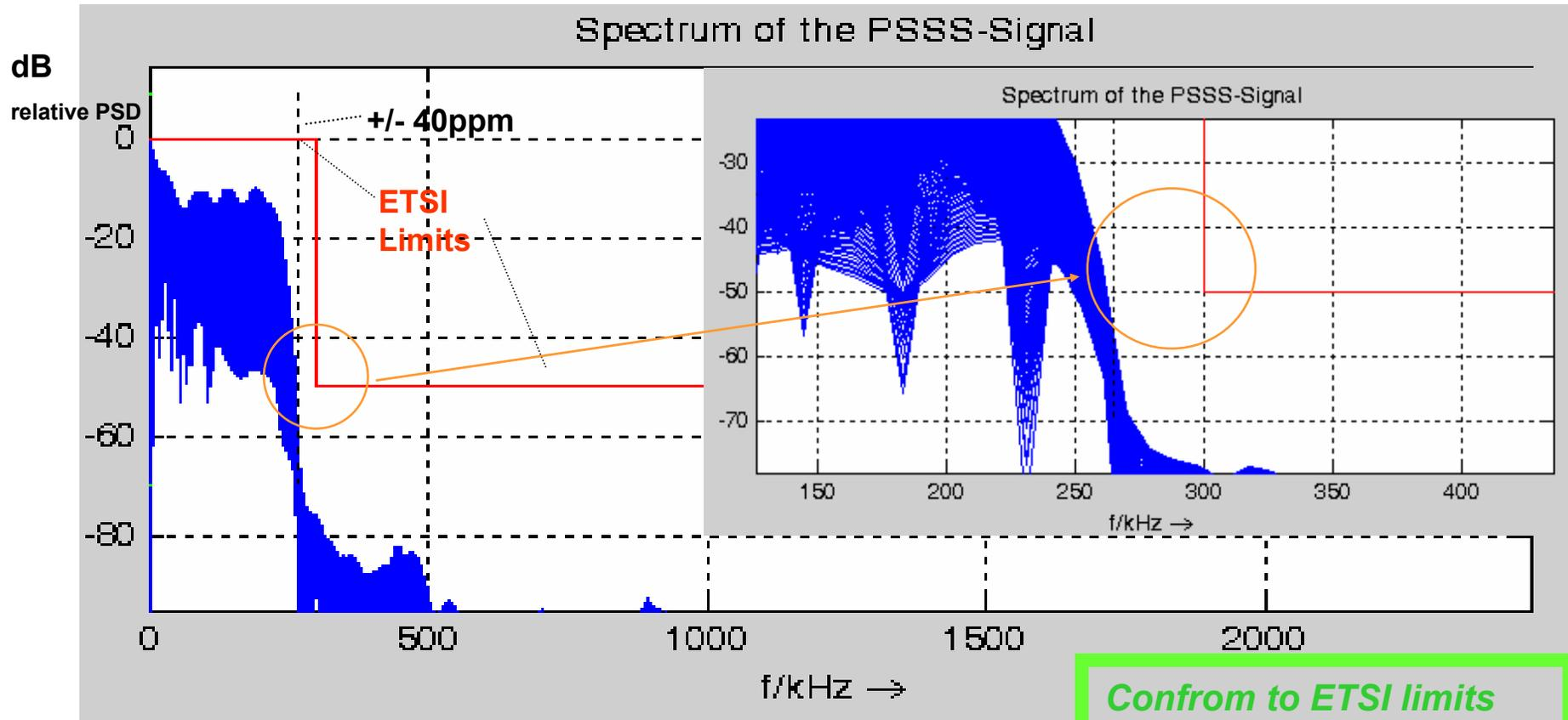
Simulations of the relative PSD in dB for the PSSS signal at 450 kchips/s, 210 kbit/s,  $\pm 40\text{ppm}$ .
