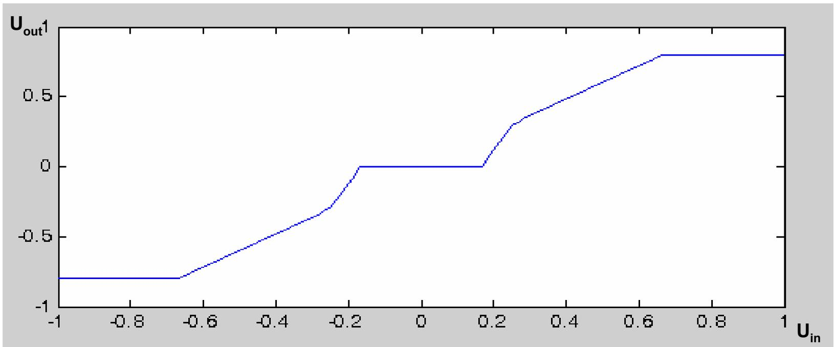
Used transfer function for simulating PSD for non linearity
