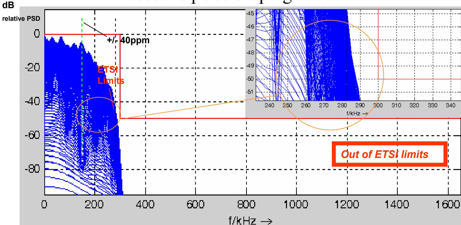
Simulations of the relative PSD in dB for the Cobi at 300 kchip/s, 150 kbit/s,  $r = 1$ , +/-40 ppm.
