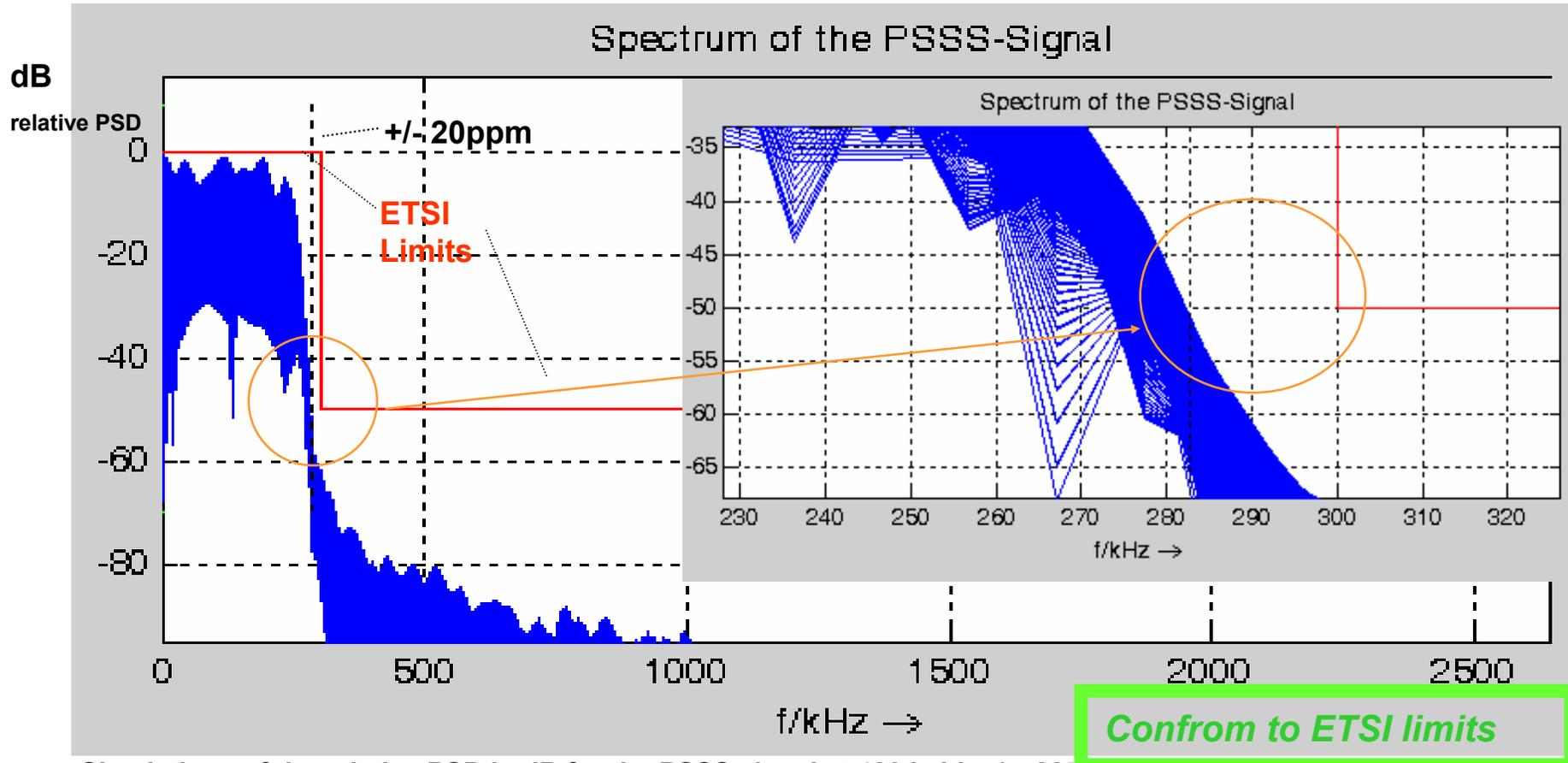
Simulations of the relative PSD in dB for the PSSS signal at 480 kchips/s, 225 kHz, +/- 20ppm.
