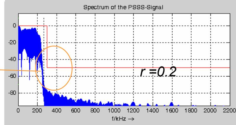
Simulations of the relative PSD in dB for the PSSS signal at 400 kchip/s 250 kbit/s.
