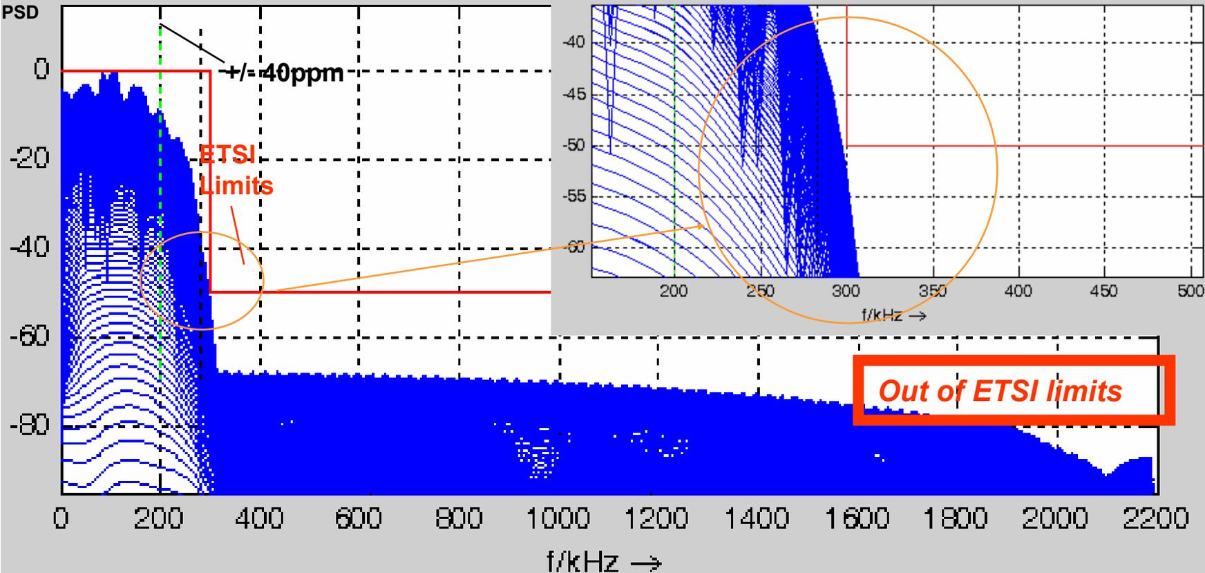
Simulations of the relative PSD in dB for the Cobi at 400 kchip/s, 200 kbit/s,  $r = 0.5$ , +/-40 ppm.
