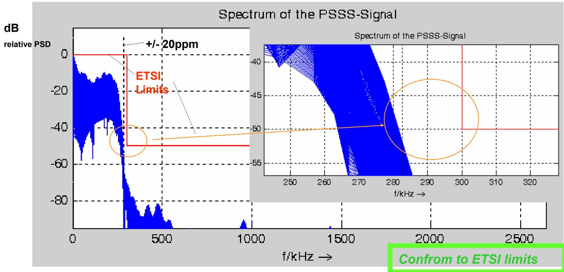
Simulations of the relative PSD in dB for the PSSS signal at 480 kchips/s, 225 kbit/s, +/- 20ppm.
