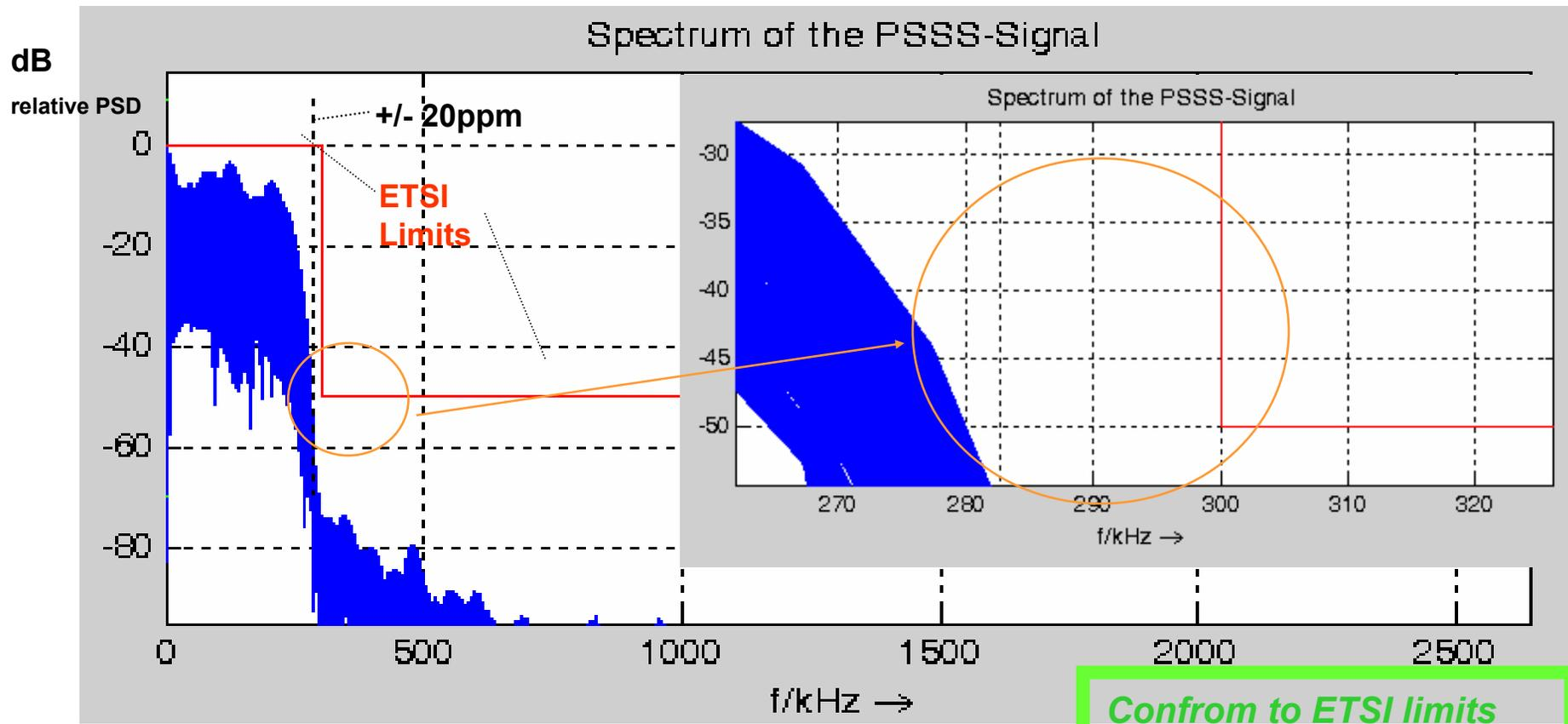
Simulations of the relative PSD in dB for the PSSS signal at 480 kchips/s, 225 kbit/s,  $\pm 20\text{ppm}$ .
