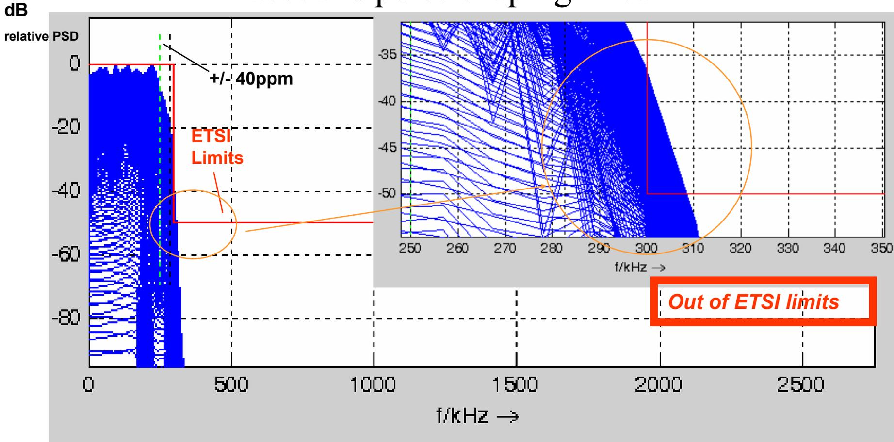
Simulations of the relative PSD in dB for the Cobi at 500 kchip/s, 250 kbit/s,  $r = 0.2$ ,  $\pm 40$  ppm.
