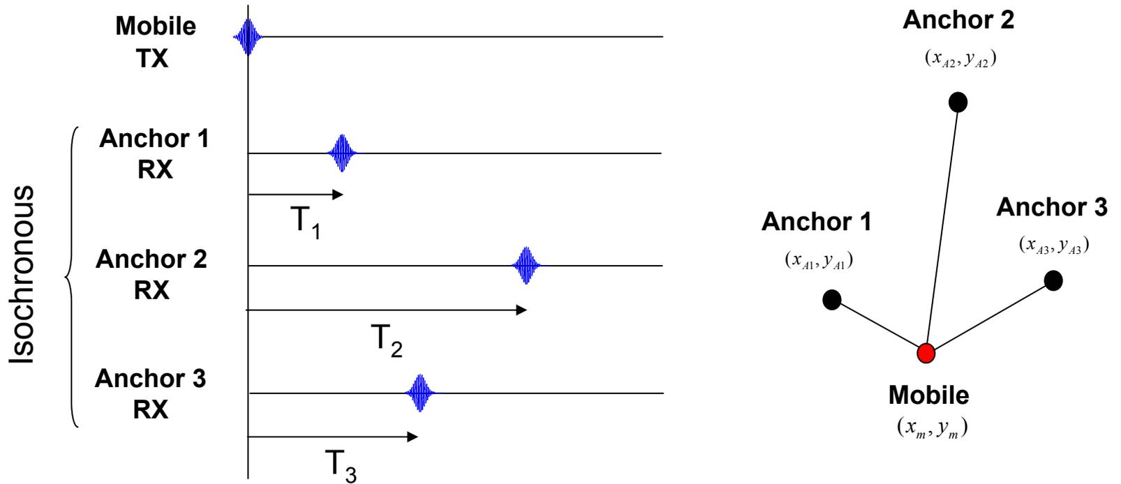
$$c(T_2 - T_1) = \sqrt{(x_{A2} - x_m)^2 + (y_{A2} - y_m)^2} - \sqrt{(x_{A1} - x_m)^2 + (y_{A1} - y_m)^2}$$
