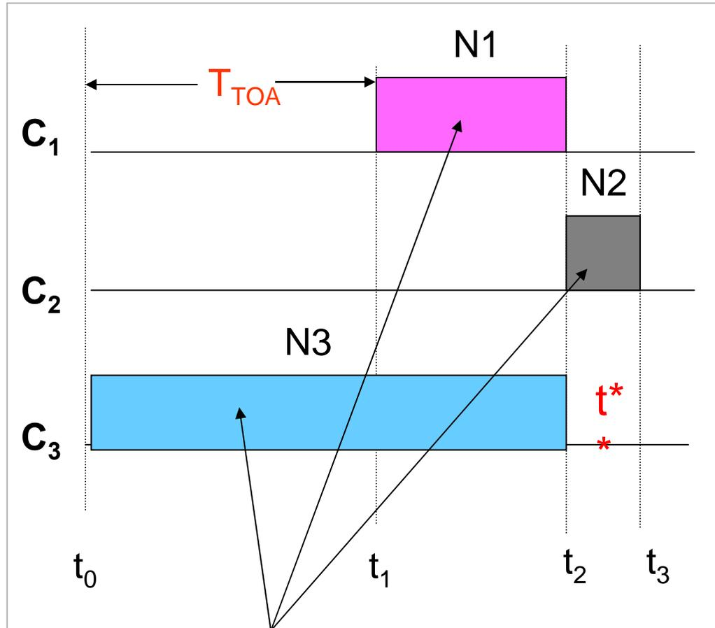
Operation time of counters  $C_1$ ,  $C_2$ ,  $C_3$ .
