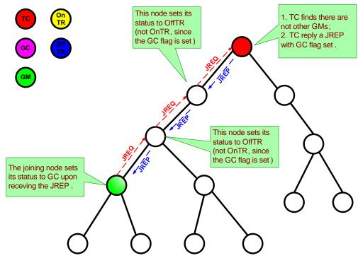
Figure 3. Joining case 1 – the first GM joins
