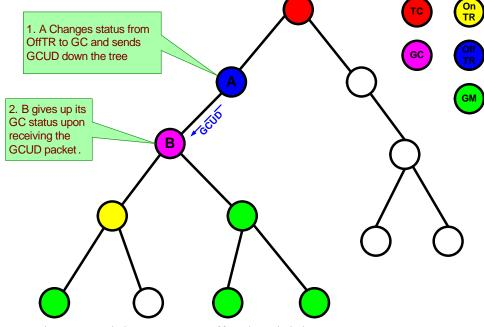
Figure 4. Joining case 2 – OffTR/GC joining
