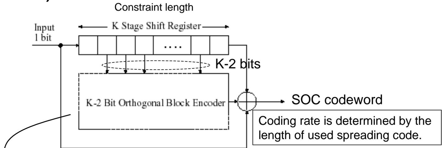
Figure 1: Encoder for SOCC of arbitrary constraint length  $K$ .
