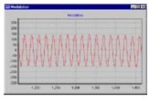
Figure 3. Parts of the payload during a frequency offset measurement where each 1 and 0 in the received payload is over-sampled 9 times. The used payload is 0101010<sup>1</sup>.
