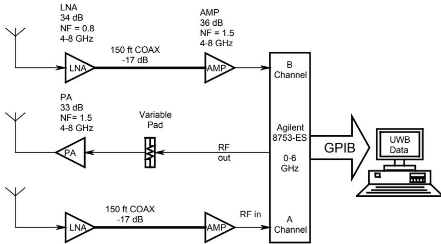
Figure 1: Channel Sounder Transceiver
