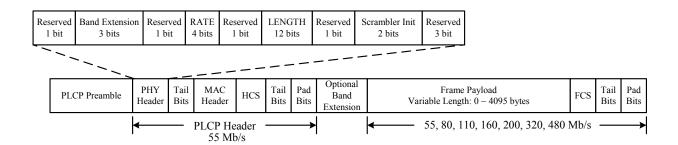
Figure 2 – PLCP frame format for a Mode 1 device
