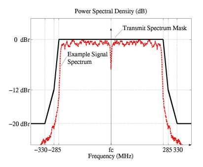
Figure 17 – Transmit Power Spectral Density Mask
