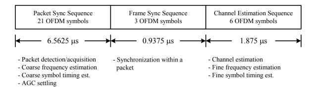
Figure 23 – Timeline for acquisition of the standard PLCP preamble
