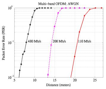
Figure 24 – PER for a Mode 1 DEV as a function of distance and information data rate in an AWGN environment.
