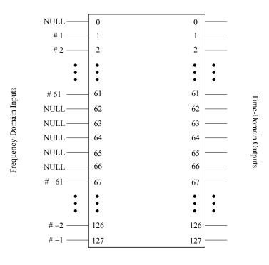
Figure 1 – Input and outputs of IFFT
