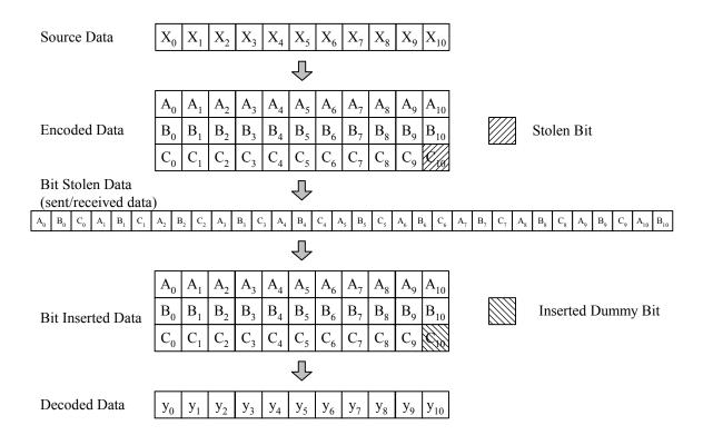
Figure 8 – An example of the bit-stealing and bit-insertion procedure (R = 11/32)
