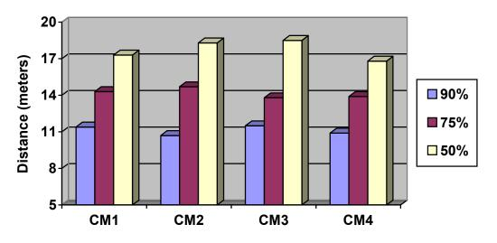
Figure 29 – Range as a function of link success probability and channel environment for an information data rate of 110 Mbps for Mode 1 (3-band) devices.
