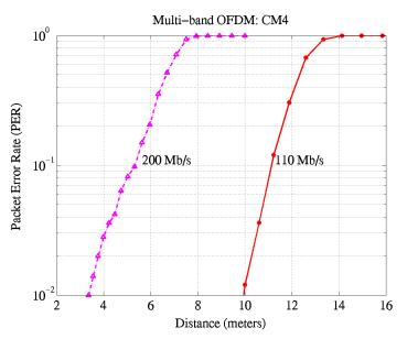
Figure 28 – PER for Mode 1 Devs as a function of distance and information data rate in a CM4 channel environment for the 90<sup>th</sup> %ile channel realization.
