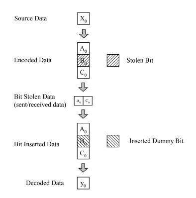
Figure 9 – An example of the bit-stealing and bit-insertion procedure (R = 1/2)
