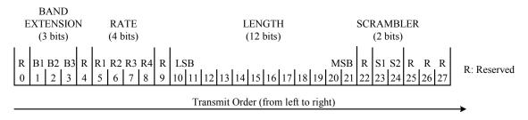
Figure 5 – PLCP Header bit assignment
