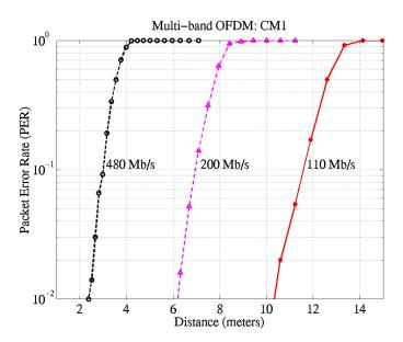
Figure 25 – PER for Mode 1 DEVs as a function of distance and information data rate in a CM1 channel environment for the 90<sup>th</sup> %ile channel realization.
