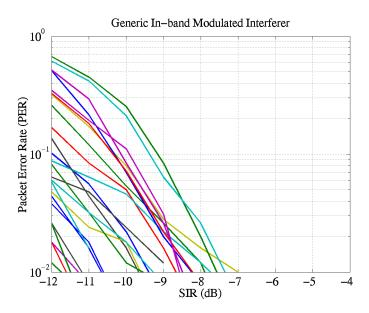
Figure 18: PER performance in the presence of a generic in-band modulated interferer
