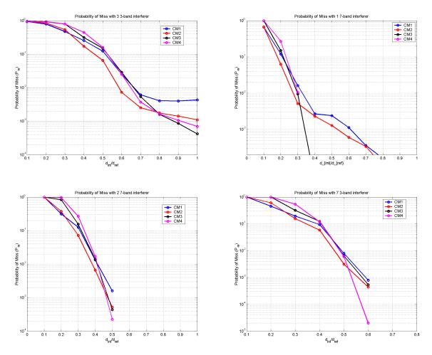
Figure 21 – Probability of miss detection versus separation distance and varying number of 3-band and 7-band interferers.
