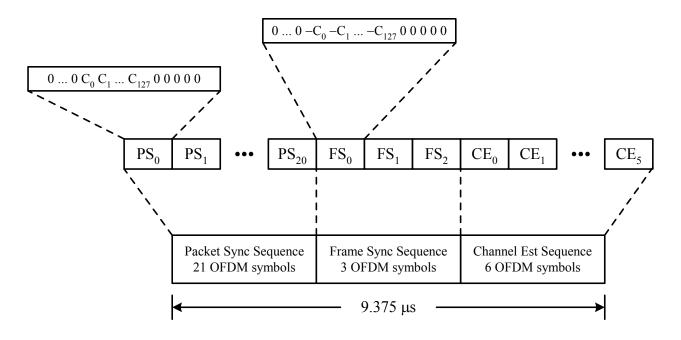
Figure 3 – Standard PLCP preamble format
