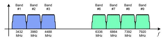
Figure 15 – Frequency of operation for a Mode 2 device.
