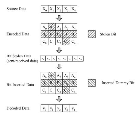
Figure 10 – An example of the bit-stealing and bit-insertion procedure (R = 5/8)
