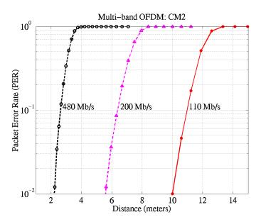
Figure 26 – PER for Mode 1 DEVs as a function of distance and information data rate in a CM2 channel environment for the 90<sup>th</sup> %ile channel realization.
