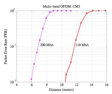
Figure 27 – PER for Mode 1 DEVs as a function of distance and information data rate in a CM3 channel environment for the 90<sup>th</sup> %ile channel realization.
