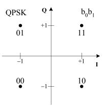
Figure 12 – QPSK constellation bit encoding
