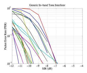
Figure 19: PER performance in the presence of a generic in-band tone interferer
