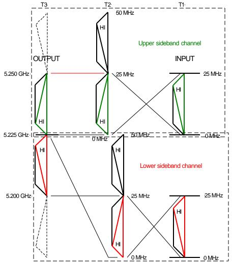
Figure A-1 Frequency relationship diagram for transmit conversion steps
