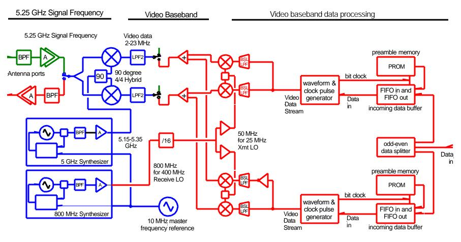
Figure A-2 5.25 GHz dual ISSB AM data radio transmitter block diagram (60 Mbps in 48 MHz bandwidth)
