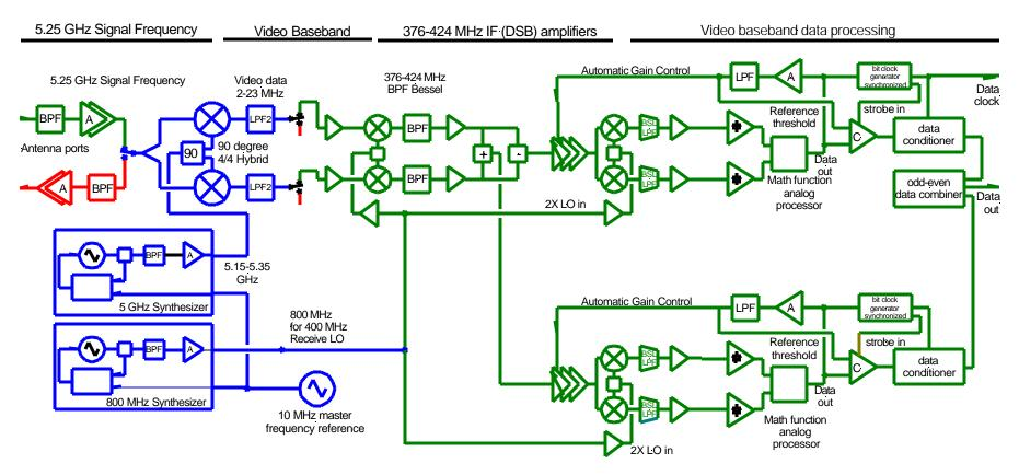
Figure A-3 5.25 GHz dual ISSB AM radio receiver block diagram
