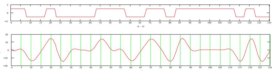
Figure 1 Data stream and associated 3-level analog waveform
