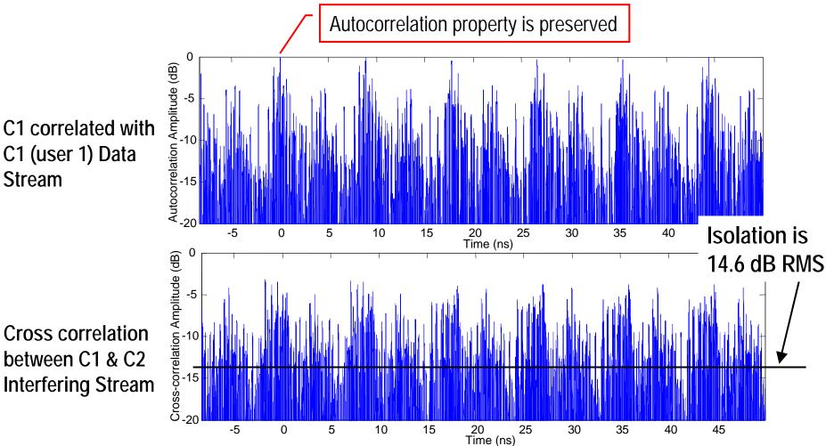
Isolation is 14.6 dB RMS – Only 2.5 dB off of clear channel Demonstrable Robust Multi-User Performance in Multipath
