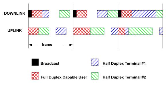
FIGURE 2. Example of Burst FDD Bandwidth Allocation
