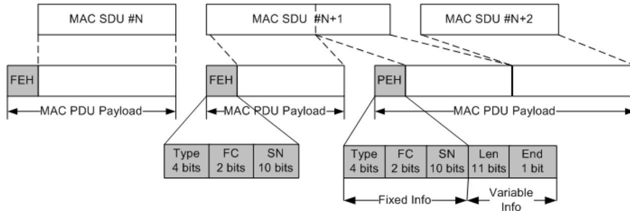
\* if 'n' SDU/SDU fragments are packed in MPDU payload then (Len, End) fields are added 'n-1' times in FPEH
