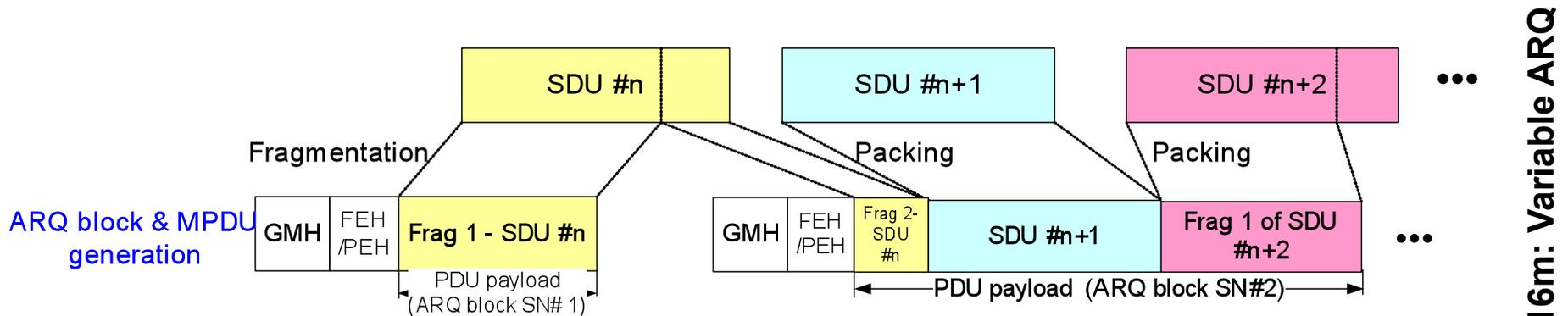
Figure.2. 16m ARQ block and MPDU generation for Initial transmission
