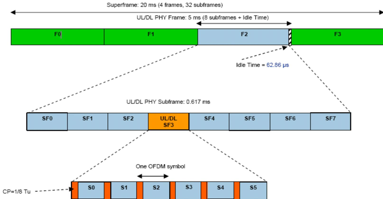
Figure 18 Frame structure with type-1 subframe in FDD duplex mode ( $CP=1/8 T_u$ )
