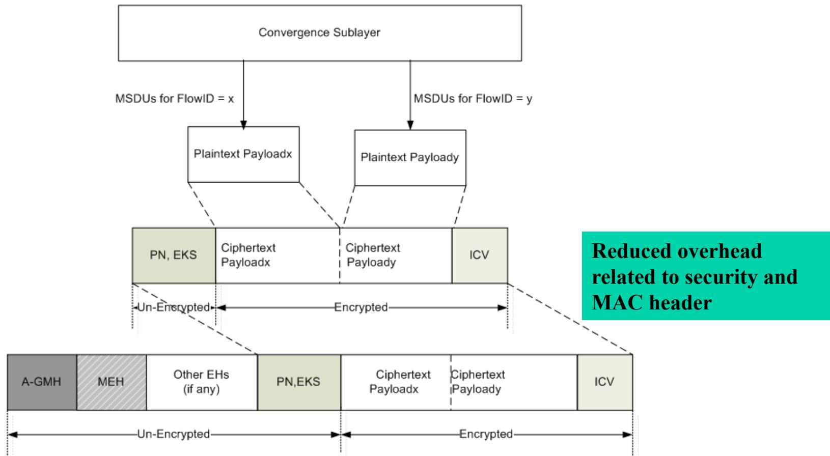
Multiple connections' payload associated with same security association are multiplexed and encrypted together in a MAC PDU.
