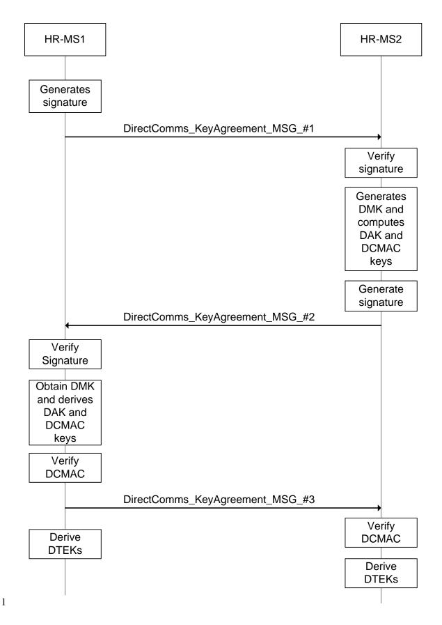
Figure 808—Flow Diagram of Authentication and Key Establishment of Direct Communication without Infrastructure (HR-MS becomes HR-BS\*case).
