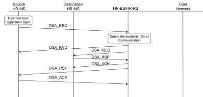
Figure 802—The establishment of direct communication between HR-MS
