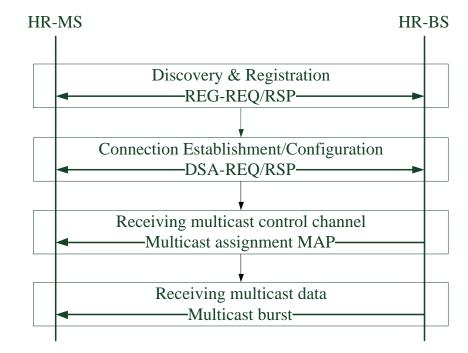
2 Figure 804 – Procedure of multicast communication establishment
