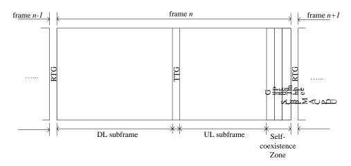
Figure 811—TDD frame structure with self-coexistence zone.
