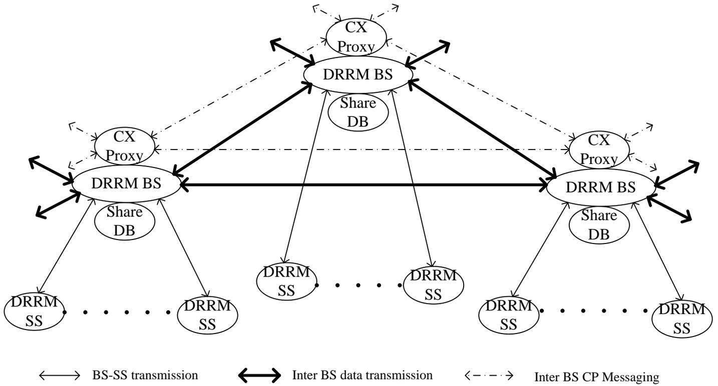
**Figure h18a – System Architecture type 2**
