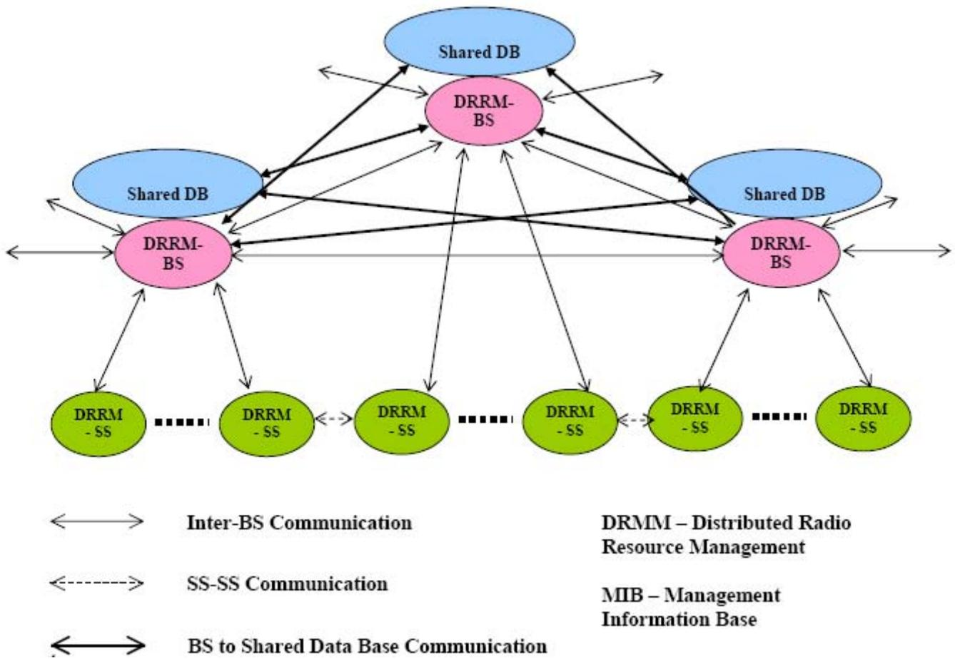
Figure 18 – System Architecture type 1
