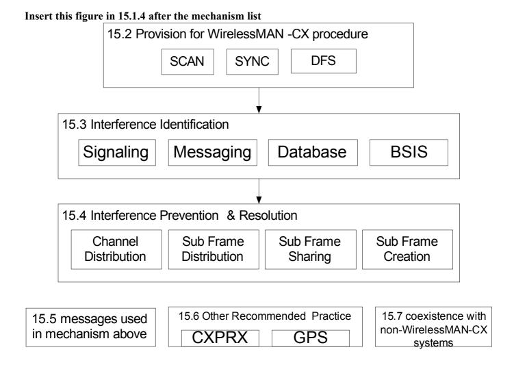
Note 1: The radio signaling mechanisms are defined in order to provide the basic connectivity information between neighbor systems using different PHY profiles.
